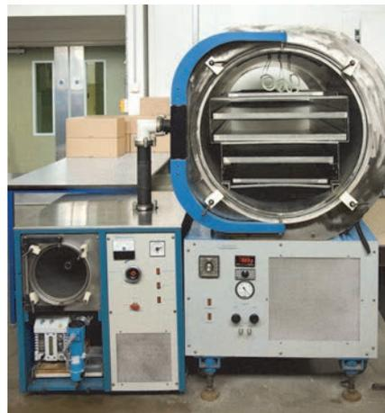
*Fig 10: Vacuum freeze dryer.*
