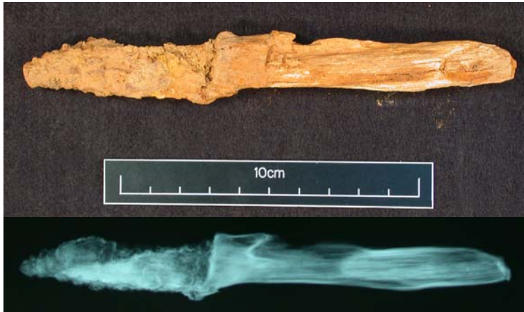
Figure 14: Iron knife SF 780 and its X-ray image.
