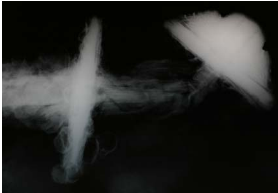
Figure 9: X-Radiograph of SF 779: pommel, hilt and guard.
