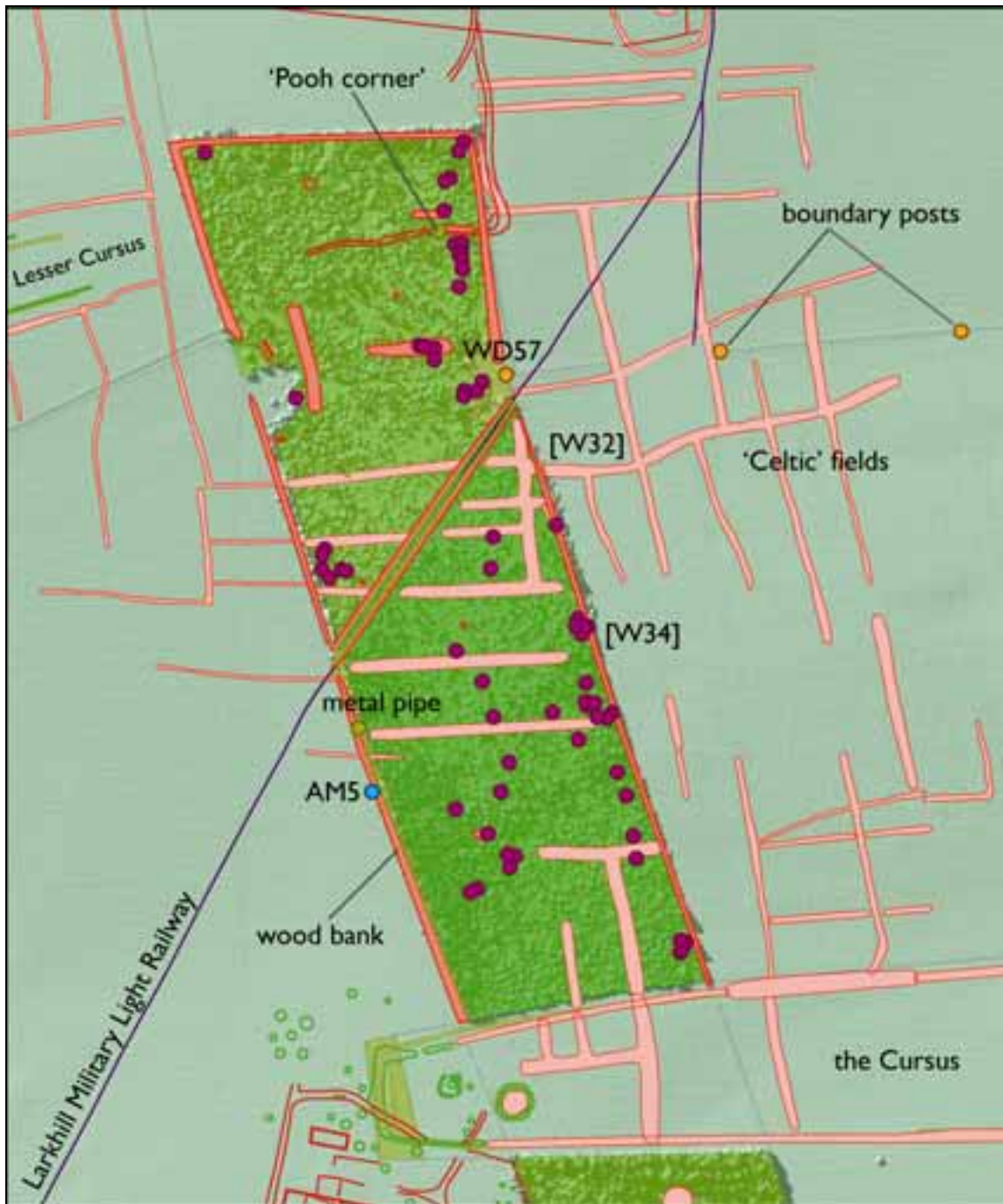
Fig 16: The 'Celtic' field system and rapid survey results at Fargo Plantation. The Level 1 survey results are shown at 1:5000 against NMP mapping and a Lidar hillshade background. The purple dots are the foxholes and the surveyed banks (in red) are shown darker than those mapped from aerial photographs and lidar. The base map is © Crown Copyright 2011. All rights reserved. Ordnance Survey Licence number 100024900. Lidar © Environment Agency (December 2001).
