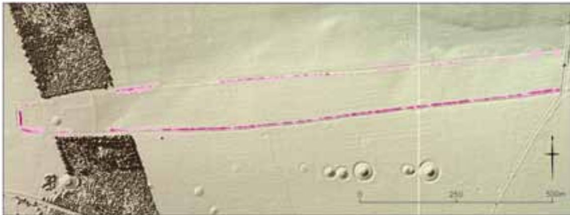
Figure 11. Ground model of the Stonehenge Cursus west of the by-way to Larkhill. The model is derived from 3D data recorded during the field survey and is coloured to show variations in the height of the bank from 0.1 to 0.5m relative to the natural ground level (darker = higher).
