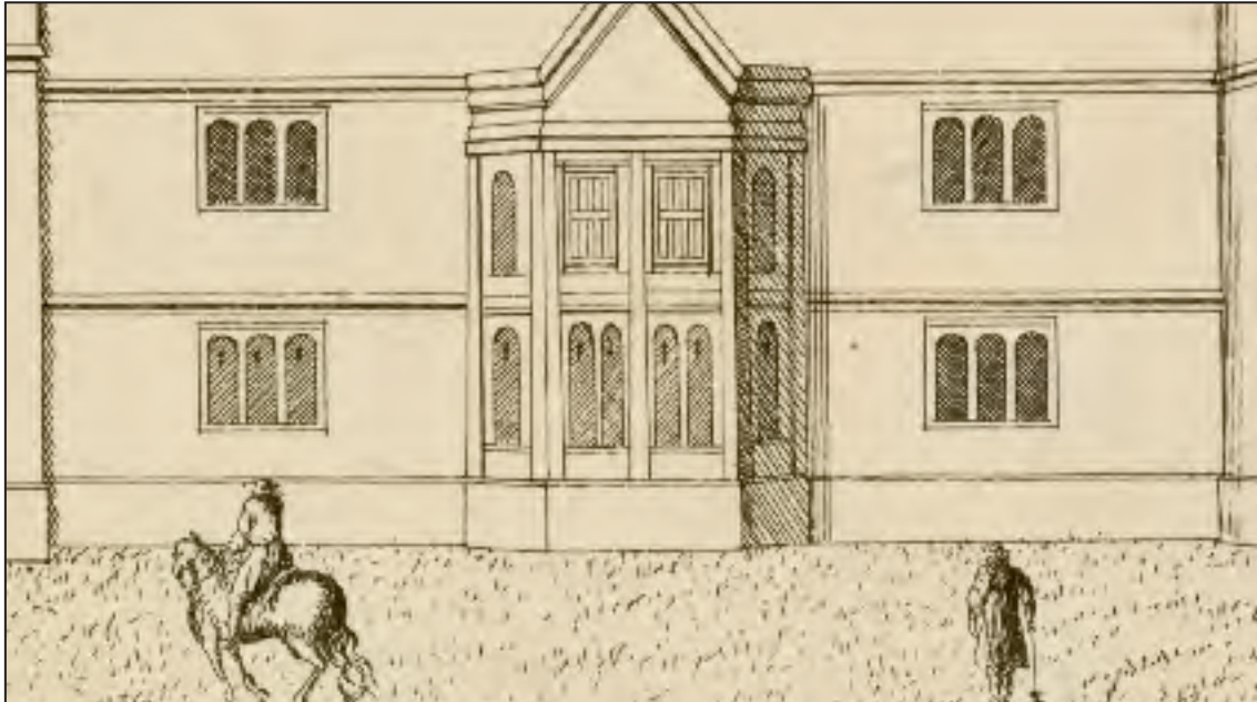
Figure 30. Henry Winstanley, c.1680. A detail of the north front showing the partially blocked window (bottom left) with its diagonal hatching and the small openings in its upper lights, probably indicating that it was boarded or shuttered. The unblocked windows (top left and right) are shown with cross-hatching indicating diamond-leaded casements.
