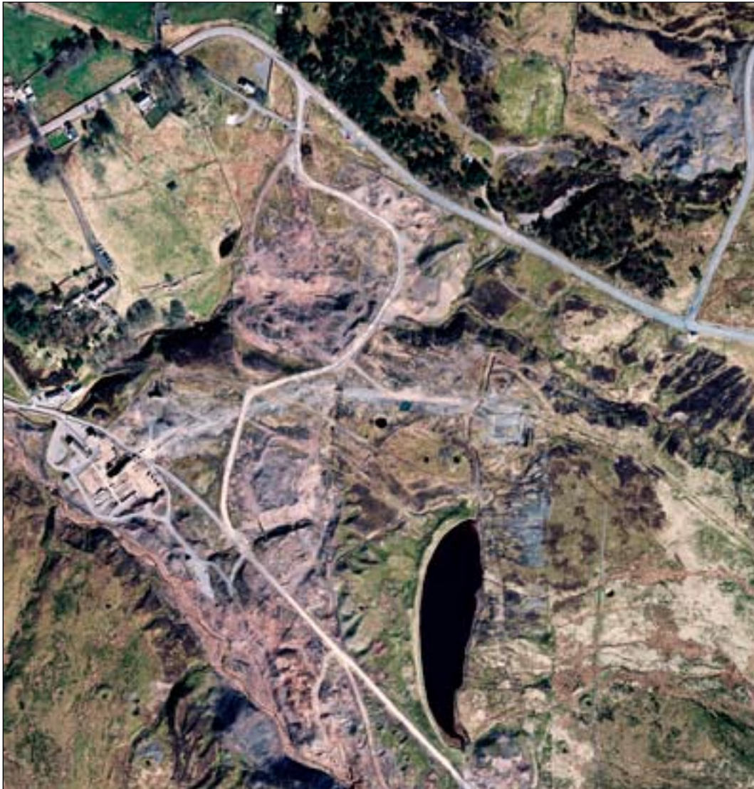
Fig 34: Lead mining remains at Nenthead highlighting the tonal differences of the lead dressing waste and spoil. Miner-Farmer Imagery NY7843 12-APR-2009
