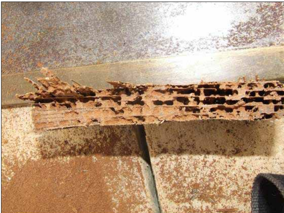
Figure 4: View of a section of a typical thatching spar showing the severe internal decay
