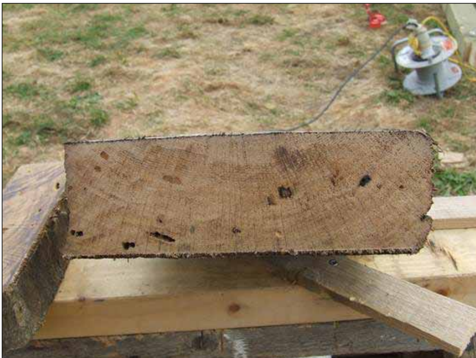
Figure 6: Cross-section of the ex-situ timber after the removal of a sample from one end
