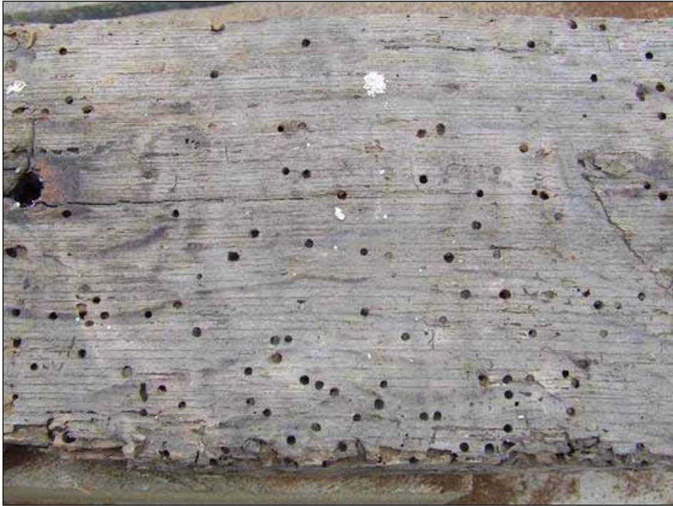
Figure 3: External view of a typical thatching spar, the grain showing a large number of rings, but also evidence of insect attack
