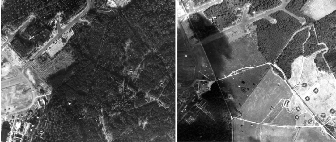
Figure 53 The bomb store at Moreton-in-Marsh. It was built in woodland to the east of the airfield and the storage bunkers are effectively concealed beneath the trees in 1947 (Left: detail of NMR RAF CPE/UK/1929 3121 16-JAN-1947) but in 1952, with the trees removed, the bunkers are easily seen (Right detail of NMR RAF 540/835 5026 14-AUG-1952)
