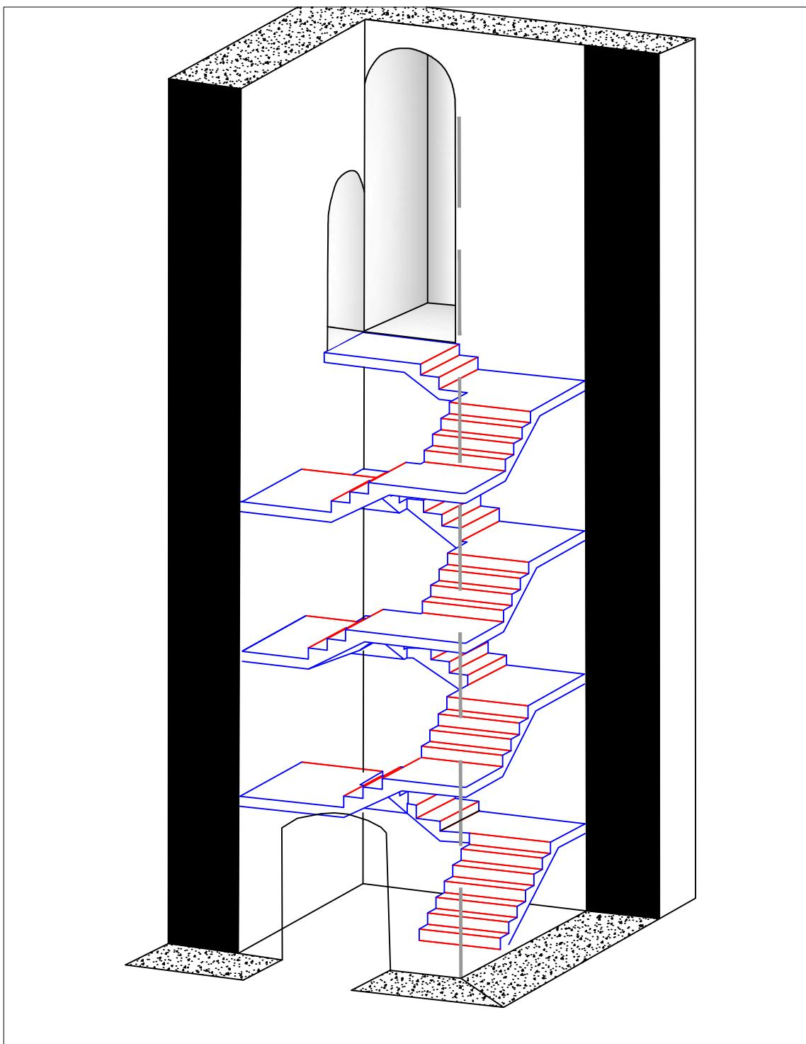
Fig 4. Isometric cut-away of stair tower viewed from the southwest, showing possible stair arrangement. Bannisters and supports omitted for clarity. Note that door at top is on the left - the archway on the right is a deep niche with solid back wall.
