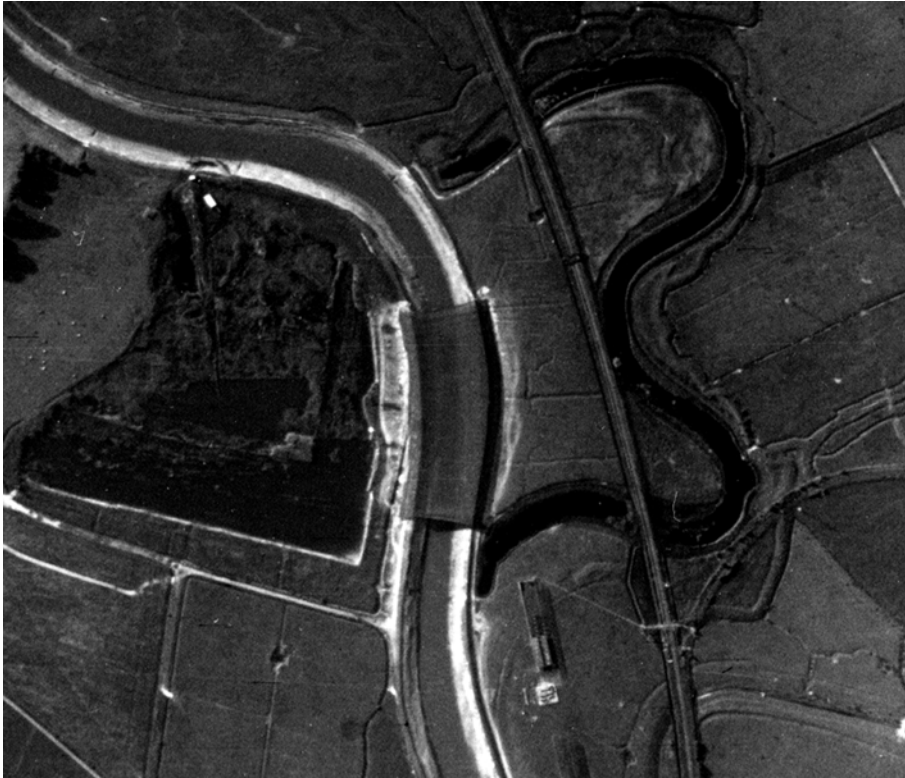
Figure 40 Camouflage netting over the River Ouse north of Newhaven. RAF HLA/600 6054 17-Jun-1942 English Heritage RAF Photography.
