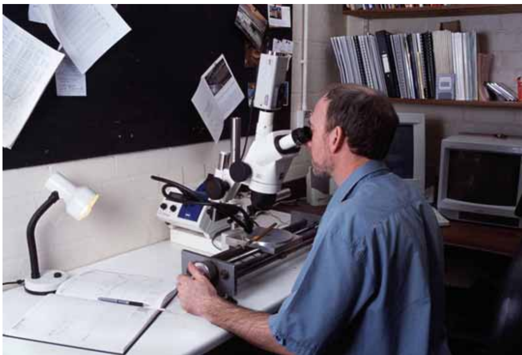
Figure A3: Measuring ring widths under a microscope. The microscope is fixed while the sample is on a moving platform. The total sequence of widths is measured twice to ensure that an error has not been made. This type of apparatus is needed to process a large number of samples on a regular basis
