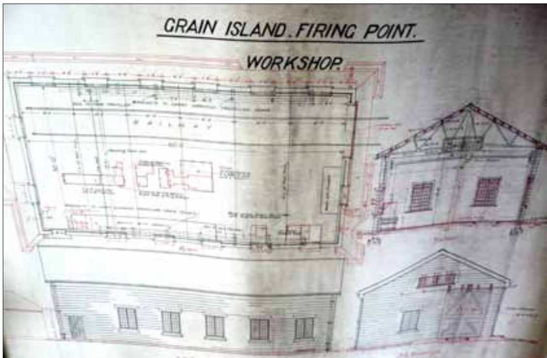
Figure 70 Detail of 1920 drawing (TNA WO 78/4370), showing the main workshop building in plan and elevation, © The National Archives.
