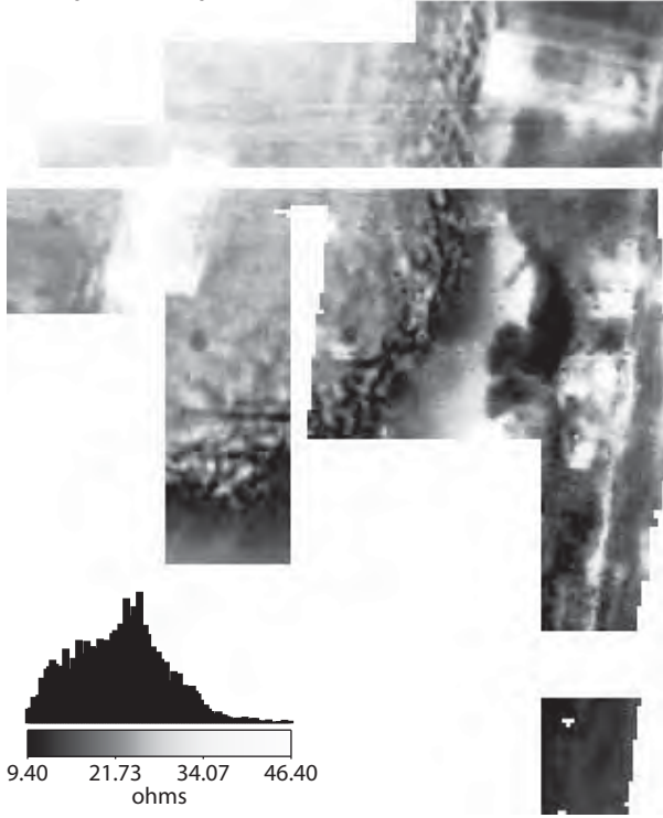
(F) Greyscale image of despiked 1.0m mobile probe separation data
