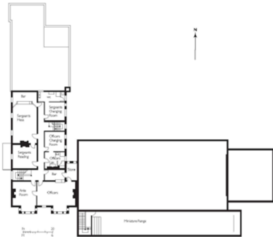
Fig 99 The plan of Peterborough's London Road drill hall as designed in 1938, showing the array of specialist rooms and facilities which were now common. © English Heritage
