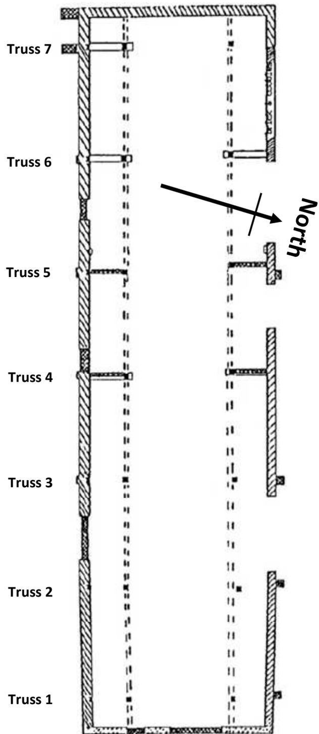
Figure 2: Plan of Hall Farm Barn, Hemsby, to show the layout and arrangement of the trusses (after John Walker)
