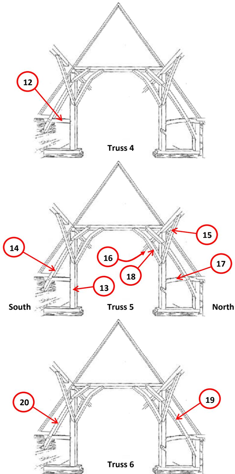
Figure 5d–f: Cross-section through the trusses to help locate sampled timbers, viewed from the east looking west (after John Walker)
