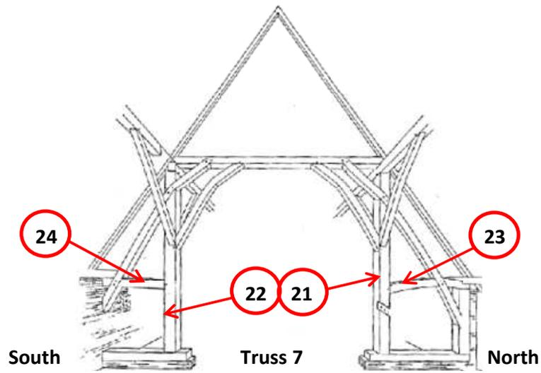
Figure 5g: Cross-section through truss to help locate sampled timbers, viewed from the east looking west (after John Walker)
