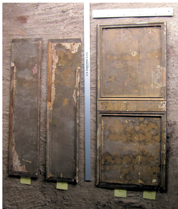
Figure 5: Medium sized boards F, G, L, and M (left to right) from Brooke House, Hackney; all grain running top to bottom (photograph Ian Tyers)
