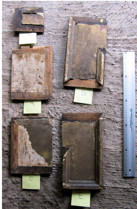
Figure 4: Smaller boards A–E from Brooke House, Hackney; all grain running top to bottom, soot presumably from fire or bomb damage still visible (photograph Ian Tyers)
