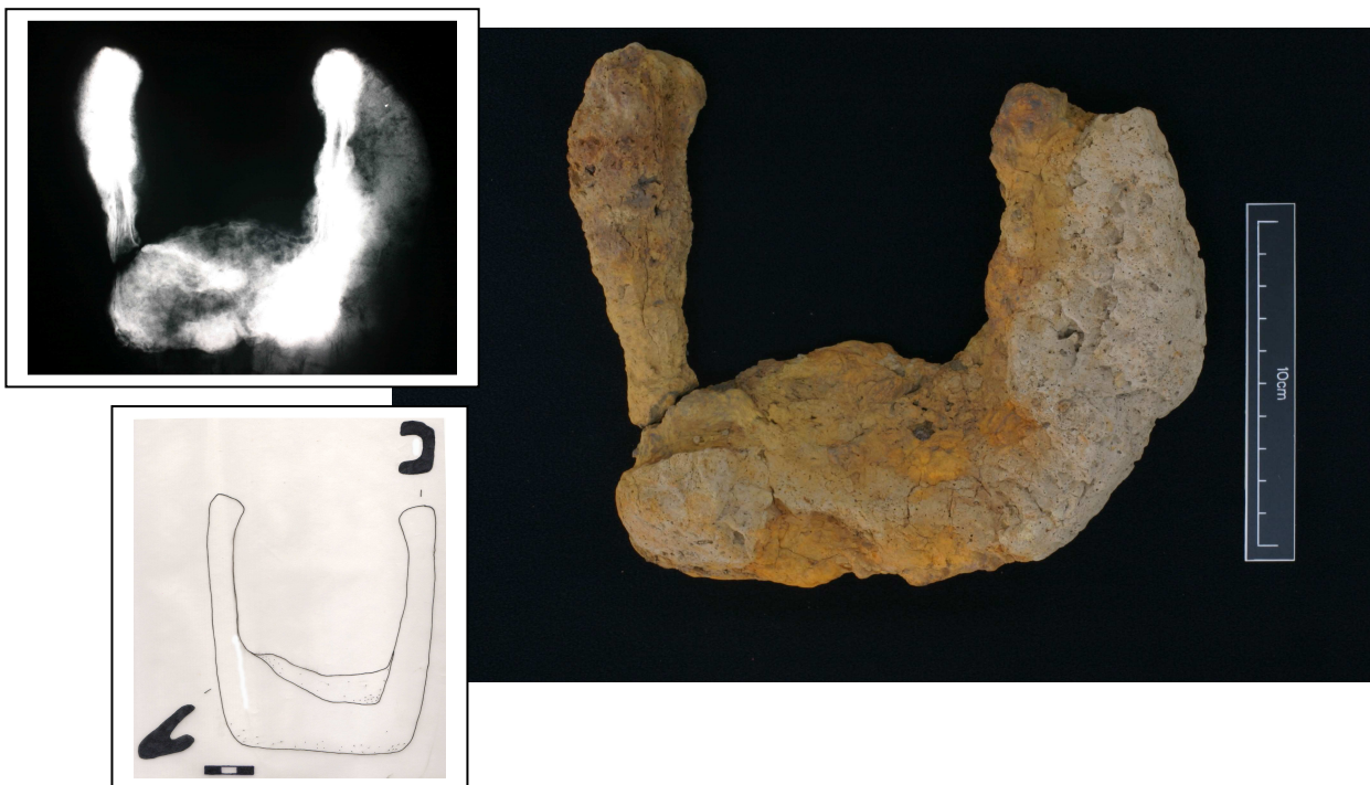
Figure 25. Spade shoe with x-ray and drawing
