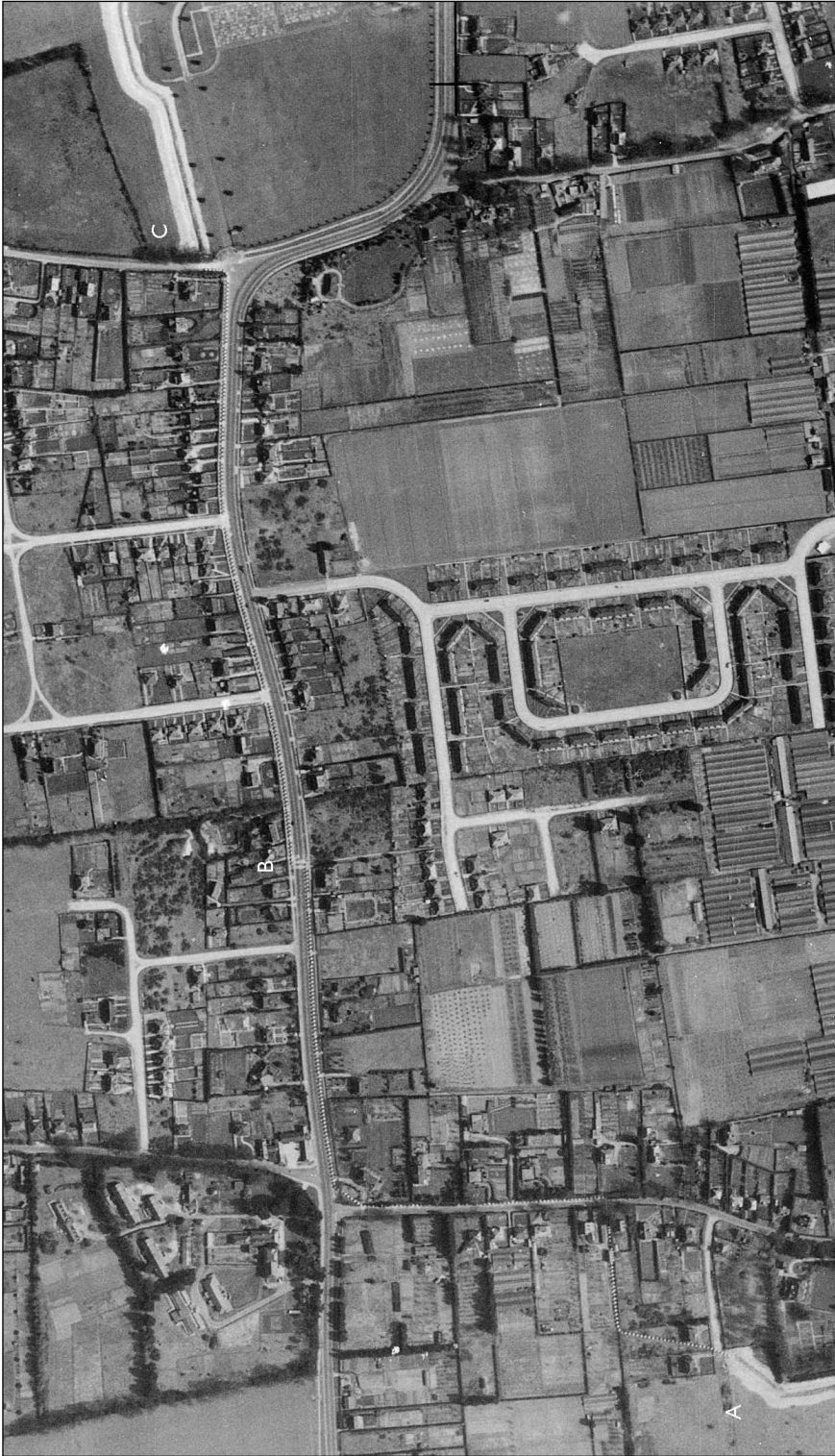
Fig 29: Part of the northern arm of the inland defence line around Worthing. The thin dark line set within a broader white one is the anti-tank ditch and can be seen lower left at A and top right, within Durrington Cemetery, at C. Between these two points can be traced a line of anti-tank cubes. The course of this line changes from one side of the A27 to the other at B and there is evidence of a road block at this point. RAF HLA/430/IPRU 6022 26-Mar-1942
