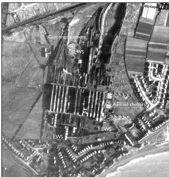
Fig 22: The Southern Railway carriage works at Lancing. There are three Emergency Water Supply (EWS) reservoirs at this site and two rows of air-raid shelters. The roof of the works has been painted with a camouflage pattern. Detail of RAF CPE/UK/1751 3054 28-Sep-1946
