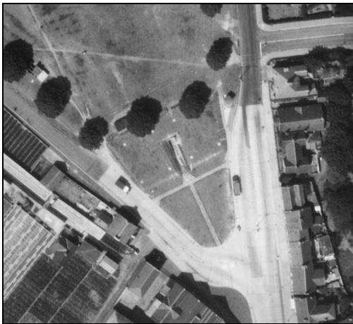
Fig 21: Public shelter situated at the south eastern corner of Broadwater Green. The shelter was entered from the south. The white circles are emergency exits. Although damaged as a result of road widening, much of this shelter still survives. Detail of RAF 58/81 5300 28-Jul-1948
