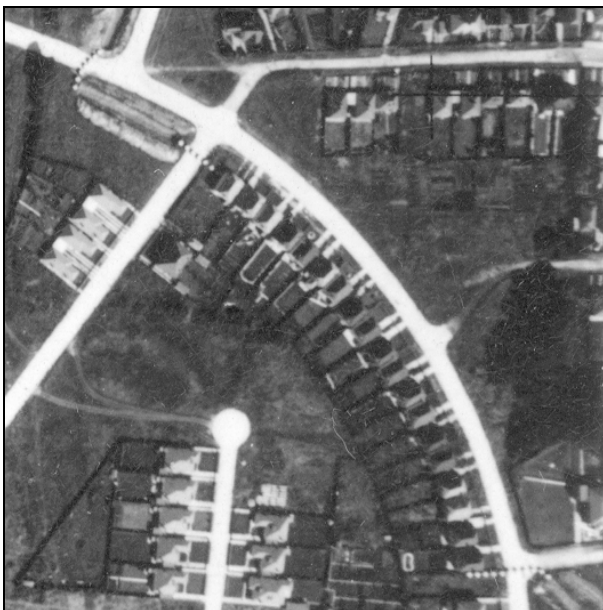
Fig 30: Part of the western arm of the defences around Worthing. This is primarily defined by anti-tank ditches and cubes, both of which can be seen to the top left and bottom right of this photograph. Between these points a row of houses on Alinora Crescent has been incorporated into the defensive line.
