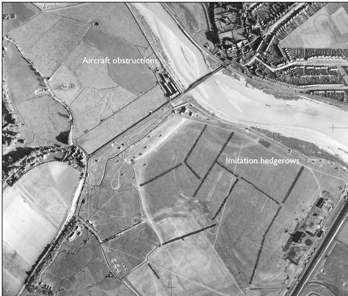
Fig 28: Shoreham airfield is at the bottom of this photograph with the terminal buildings bottom right. The dark lines are 'fake field hedgerows' that have been painted onto the ground, possibly to prevent enemy aircraft landing here, or to disguise against air attack. In the field to the north a series of banks and ditches have been dug as aircraft obstructions, sometimes known as anti-glider trenches. Their purpose was to interrupt open areas to an extent that made the landing and then take-off of enemy troop carrying aircraft impossible. Detail of RAF S 653/H9/140 027 07-Nov-1941
