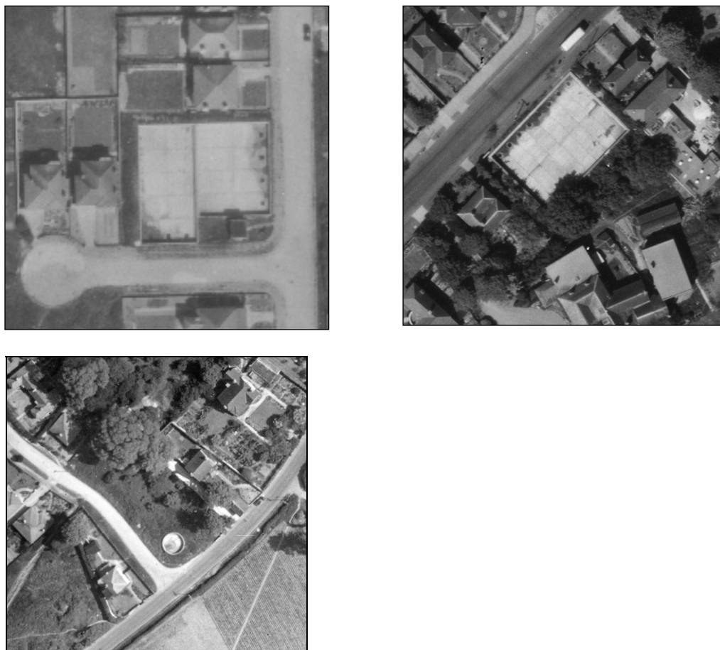
Fig 23: Various EWS photographed after the war and empty of water. The photograph top left shows two EWS in West Worthing at the junction of Anscombe Close and Anscombe Road. The possible drains are seen as dark squares along one side of each tank. The EWS top right is situated in front of what is now Broadwater Manor School and has circular drains. Bottom left is an example of a circular EWS in Lancing, at the junction of Manor Road and Griffith's Avenue.
