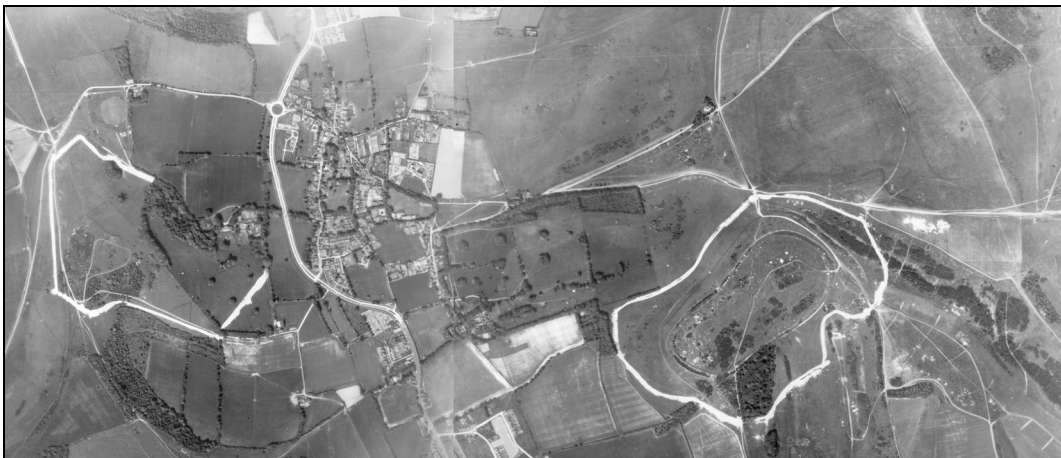
Fig 31: Findon Nodal Point. Both Cissbury Ring and Church Hill have been enclosed by an anti-tank ditch and, in places, anti-tank cubes. These two enclosures are connected to a third south of Findon.
