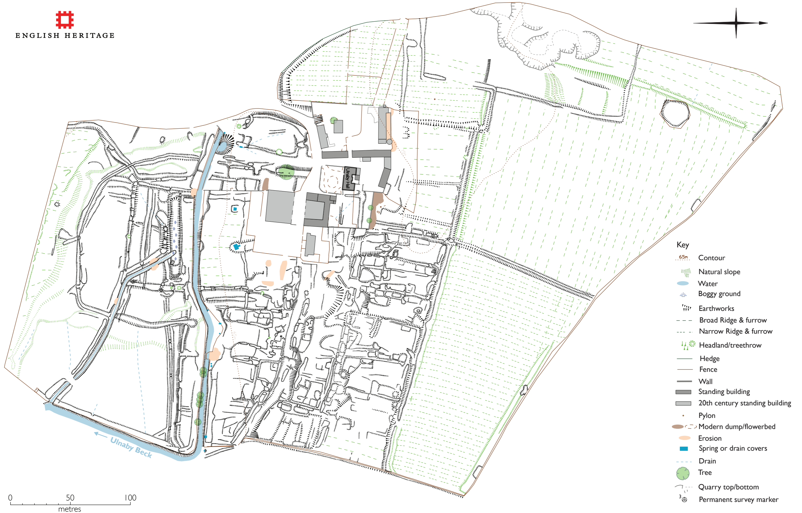
Figure 12: English Heritage plan of the earthwork remains at Ulnaby, surveyed at 1:1000 (not to scale)
