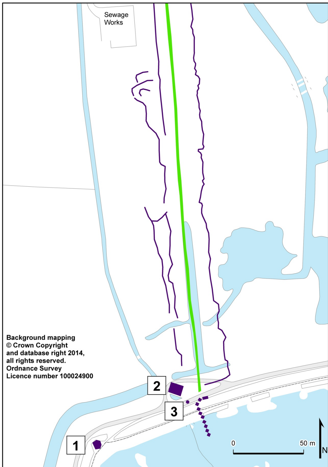
Figure 8 Air photo mapping of the stop line north from the River Medway. It comprises the anti-tank ditch (green) with flanking cleared area (extents defined by purple lines), anti-tank cubes and supporting features (purple). Numbers refer to the table below.
