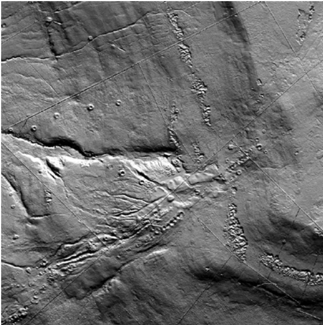
Figure 64: Sample LiDAR from the North Pennines Miner-Farmer project. Digital Terrain Model (DTM) showing the Km square NY 7443 which contains extensive mining remains. Examination of this geo-rectified data, along with digital orthophotography and field observation will provide the platform for the interpretation and recording of the extensive lead-mining landscapes in this project. © English Heritage.
