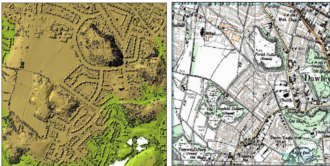
Figure 13: Remains of several coal mines at Dawley, Telford surrounded by modern housing development illustrated by the lidar tile LIDAR SJ6806 DSM 1m JAN-FEB 2011 (left) Lidar © Environment Agency copyright 2010. All rights reserved. and a composite of modern map and 1st edition OS map (right) © Crown Copyright and database right 2015. All rights reserved. Ordnance Survey Licence number 100024900
