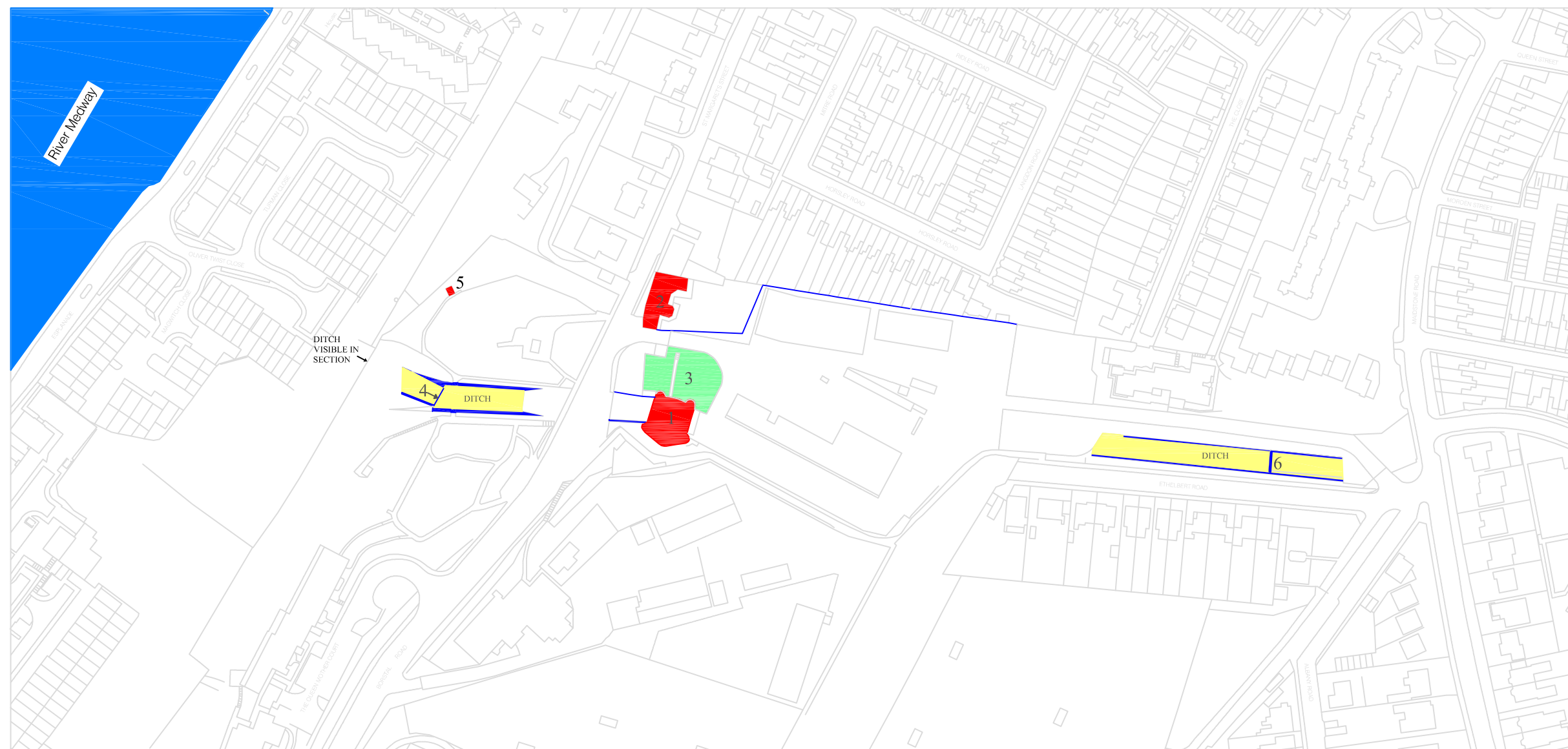
Figure 44 Map showing the surviving visible elements of Fort Clarence: 1 = Clarence Tower; 2 = The Governor's House; 3 = Earth bombproofing over the Main Magazine; 4 = West Casemates; 5 = Picquet House; 6 = Rifle butt Blue = ditch revetments and other fort walls; yellow = ditch bottom; green = earthwork; red = building (Reproduced by permission of the Director General of the Ordnance Survey)
