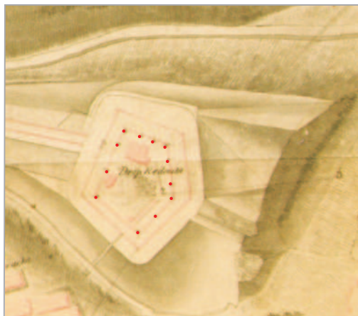
Figure 14a The Drop Redoubt in 1813, showing the terreplein gun positions, added in red by the authors (extract from PRO: MR/1/1346)
