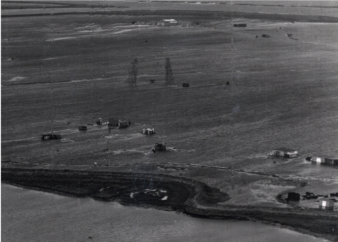
Figure 6: Photograph taken during the great flood of February 1953, showing the two steel towers between which a high explosive charge was suspended. In the foreground are scale models of various buildings, which would be subject to a blast wave when the high explosive ball was detonated. RAF 540/999 105 2 February 1953 NMR (RAF) Photography.
