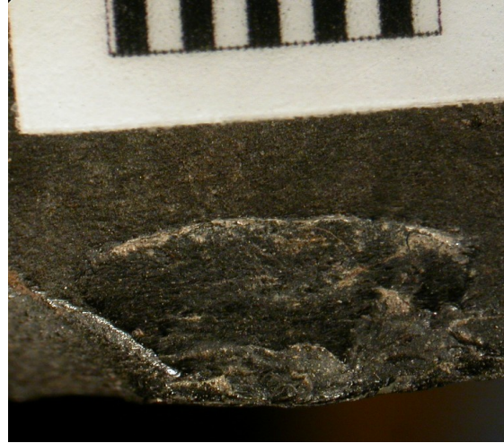
Figure 19: Jam curve on the side
