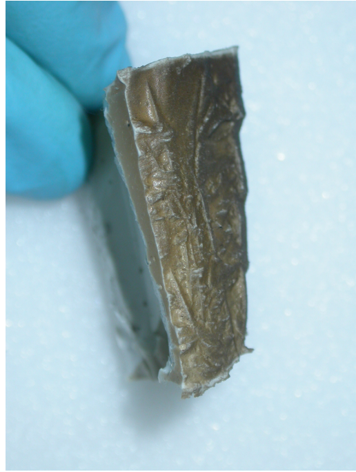
Figure 21: Step-like cross section received from gouge driven down with hammer
