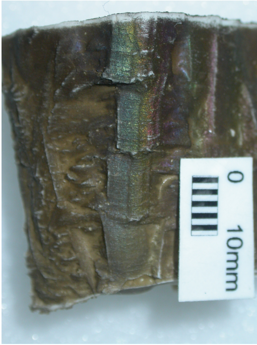
Figure 20: Silicone cast (carbon coated) illustrating pronounced stop marks
