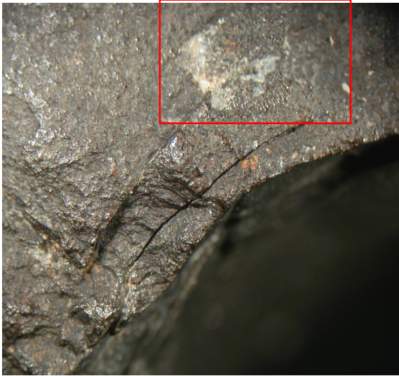
Figure 22: Fossil impression (red box) next to jam curve broken edge
