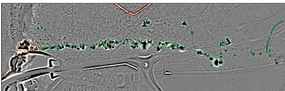
Figure 56 A linear pattern of extraction (green) visible on a lidar visualisation (LRM) within woodland on Slindon Common. Extraction of parts of the mixed quaternary deposits of clay, sand and gravel. Lidar © Copyright Fugro Geospatial and South Downs National Park Authority.
