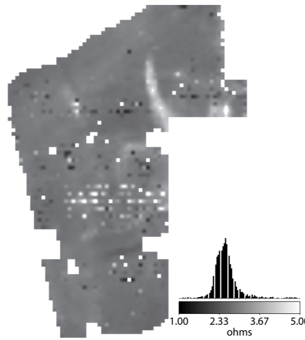
(E) Linear greyscale image of minimally processed 1.0m mobile probe separation data
