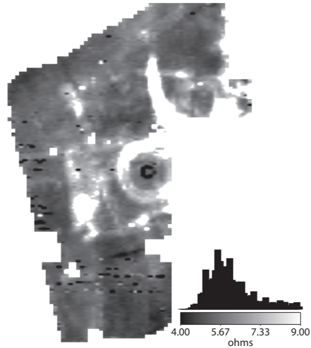
(B) Linear greyscale image of minimally processed 0.5m mobile probe separation data
