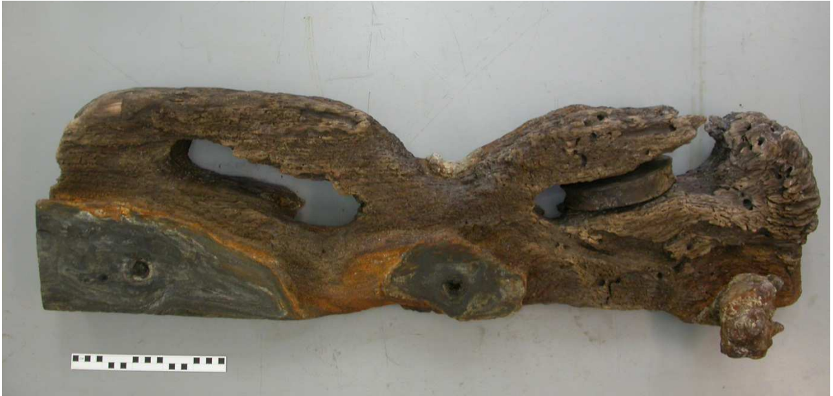
Fig 5: Fixed double block after conservation and removal of excess PEG
