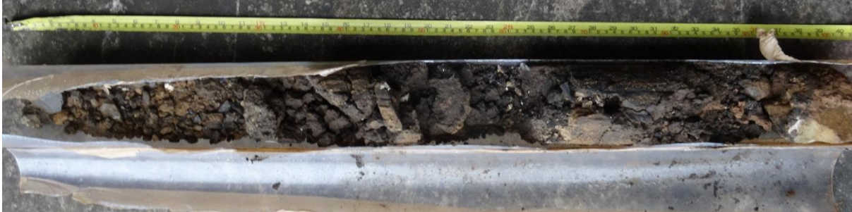
Figure 61. Borehole 10, 1.20 - 2.00 m. This appears to be 80 cm of true borehole depth spread over 100 cm of core depth; complete description therefore uses corrected figure based on this hypothesis; i.e. all depths are x 0.8. Original depths (cm) are in brackets.
