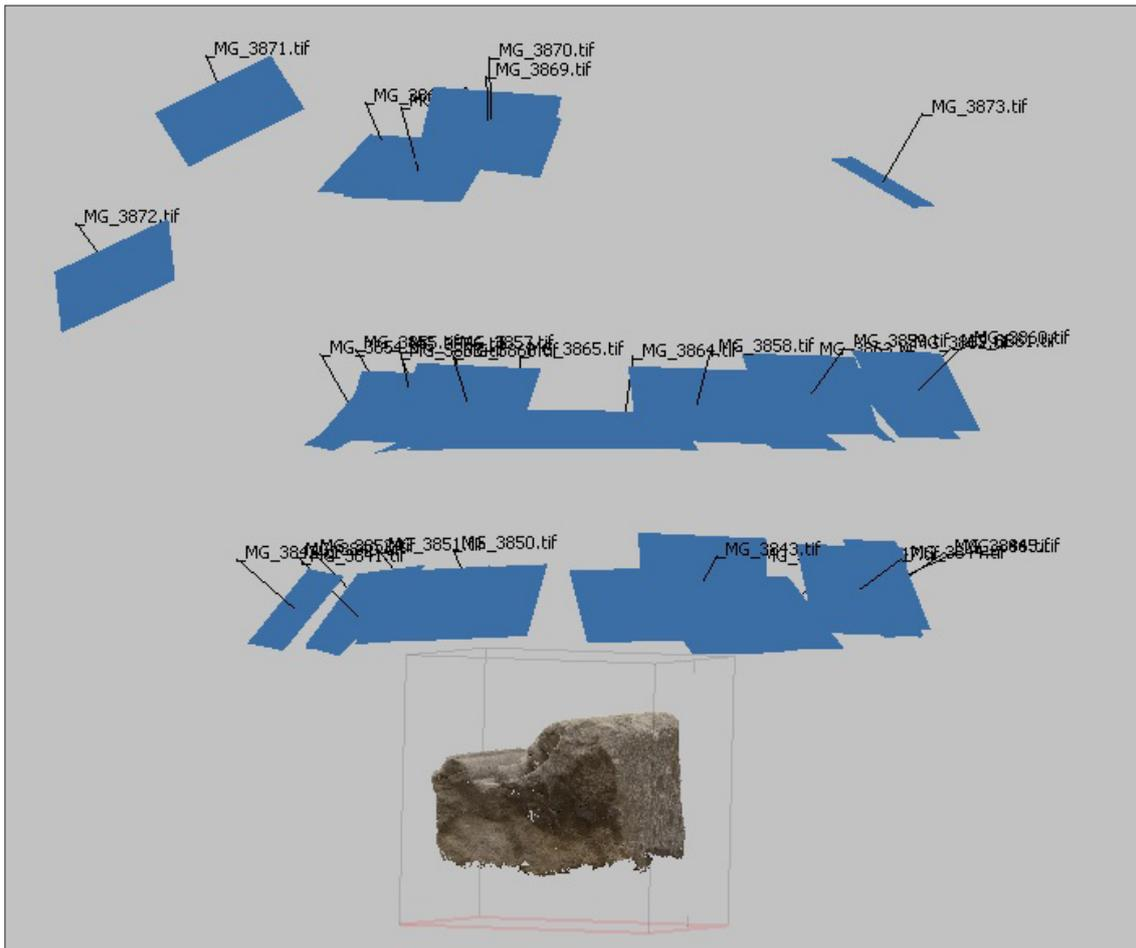
Figure 1: Screenshot from Agisoft Photoscan showing the location where each photograph was taken (blue rectangles). This view is taken from the side of the object in the 3D view port. Two circuits of photography were taken around the artefact (at the bottom) at different heights for more complete coverage, with additional shots for further details.
