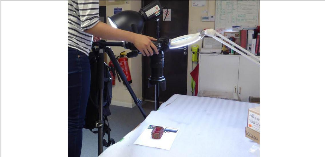
*Figure 4: The second set up for photography, using a horizontal bar on the tripod for overhead photography of the artefact and an LED lamp for lighting the artefact. The camera operator had to stand on a stool to see the artefact through the camera viewfinder.*
