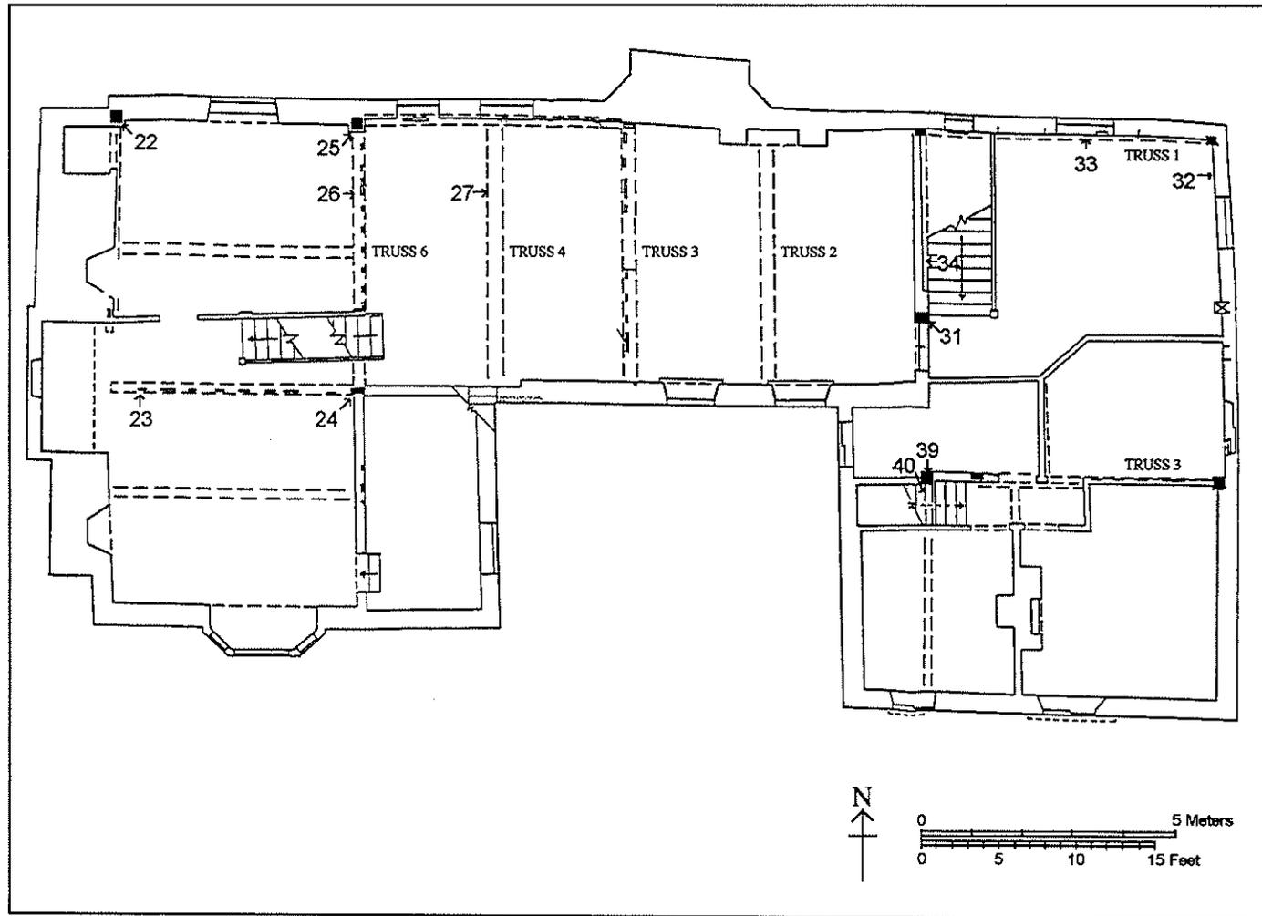
**Figure 1c:** location of samples obtained from the ground floor, Thorpe Prebend House, Ripon (after Smith 1997).
