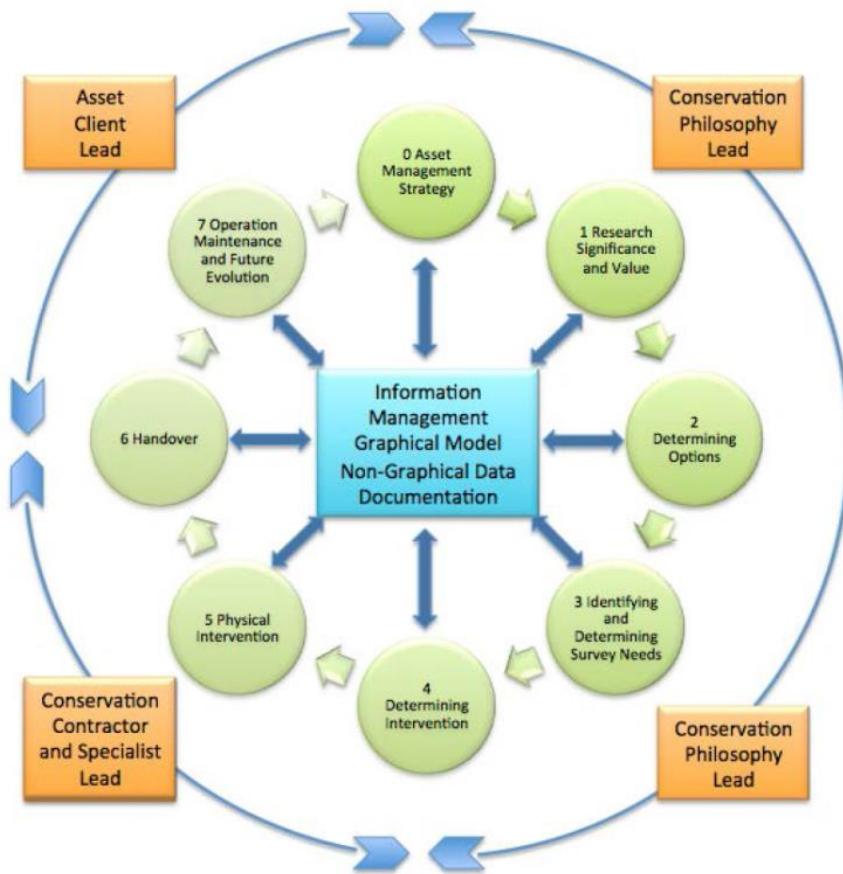
Figure 6-1 Emerging HBIM framework cyclic diagram
