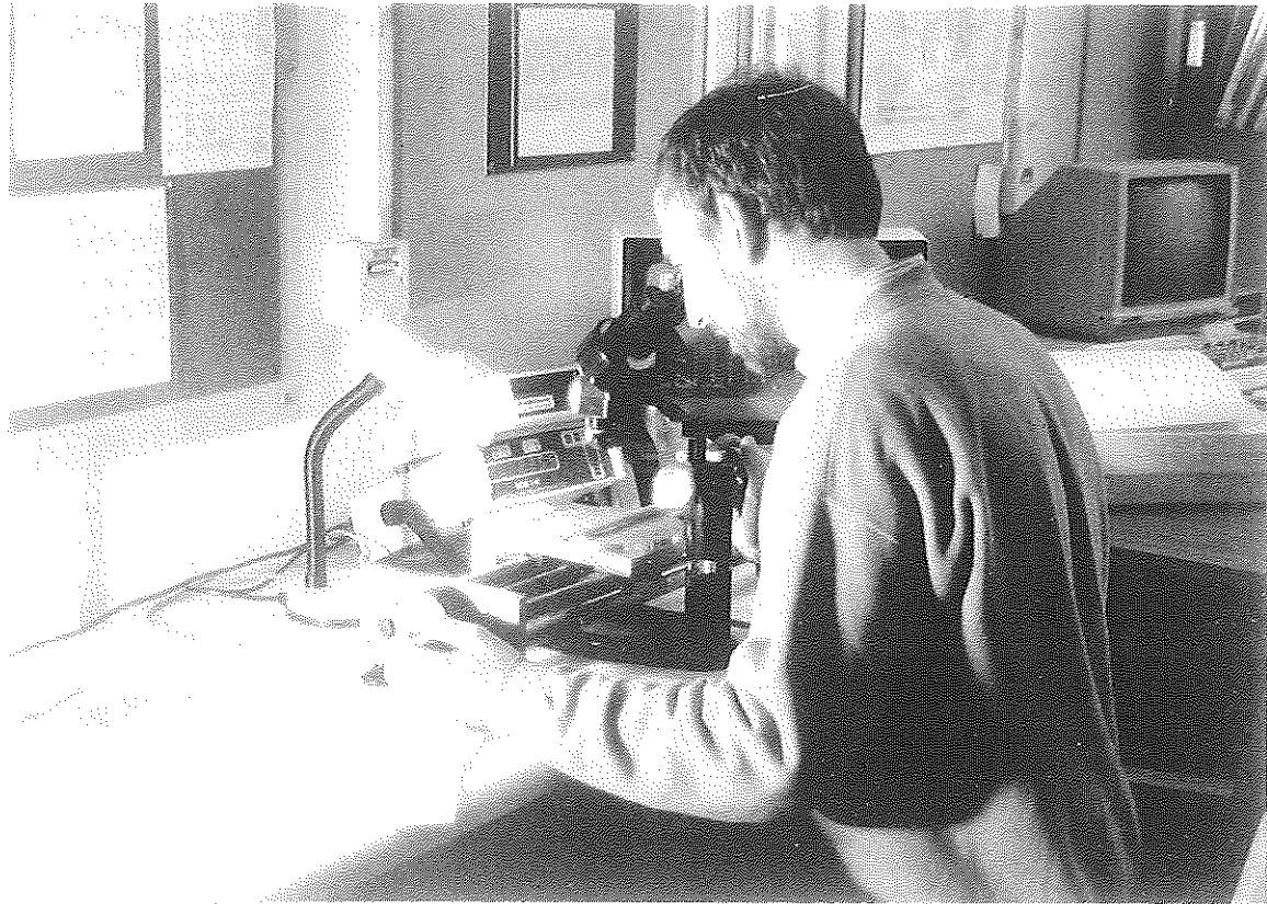
Fig 3. Measuring ring widths under a microscope. The microscope is fixed while the sample is on a moving platform. The total sequence of widths is measured twice to ensure that an error has not been made. This type of apparatus is needed to process a large number of samples on a regular basis.
