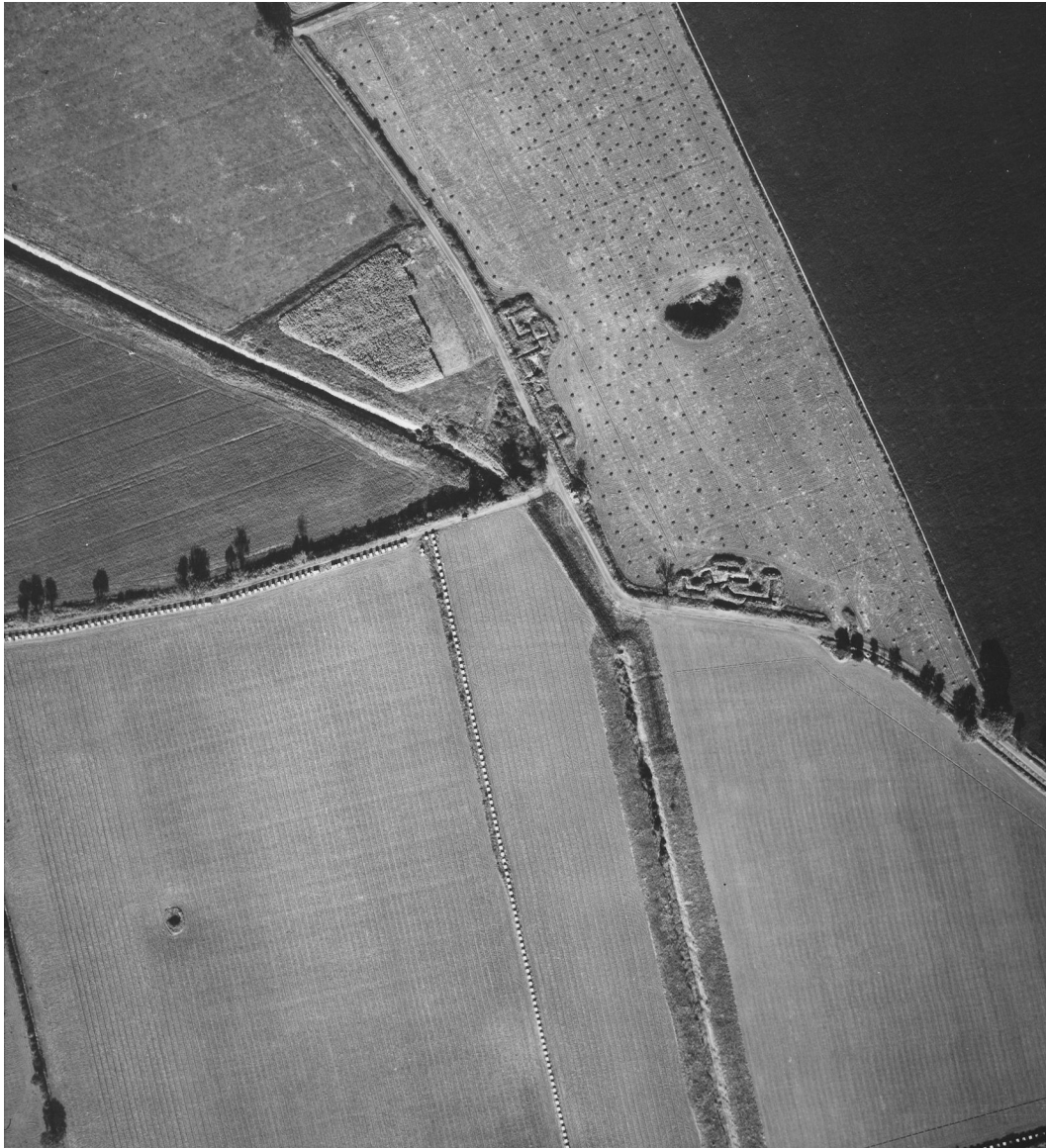
Figure 6.5. A section of the anti-tank system surrounding Lowestoft (LWT 284), showing an area of defences including anti-tank cubes, slit trenches and section posts; the latter appear to have become Forward Defended Localities (FDLs). RAF/106G/UK/927 RVp1 6033 16-OCT-1945 Historic England RAF Photography.
