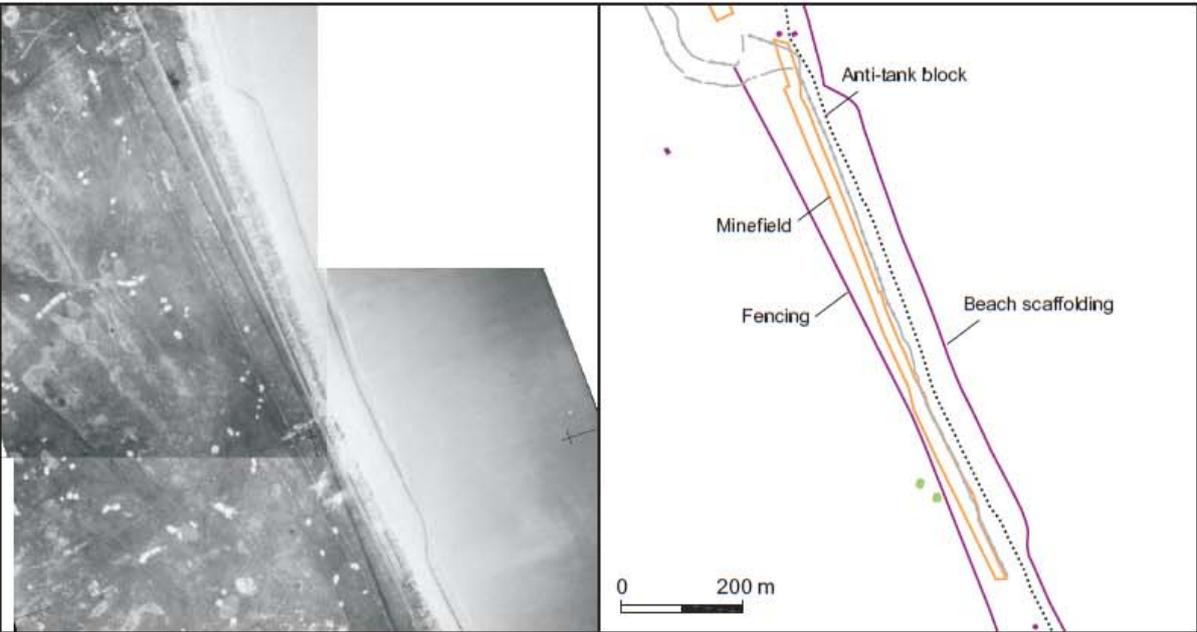
Plate 47. Anti-landing obstacles, Sandwich Flats, including a minefield, anti-tank blocks, beach scaffolding and fencing (MWX43270, Mke42015, MWX43276 and MWX43275). © English Heritage (NMR) RAF Photography
