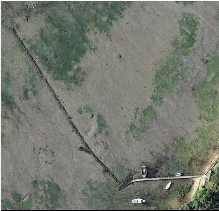
Figure 6.28: Post-medieval or early twentieth century jetty or groyne on the intertidal flats to the north of Westlands, Birdham. It is 93m long and appears to comprise a line of rubble foundation running from the end of a modern jetty directly down to the low tide mark. It is possibly the line of a eighteenth or nineteenth century jetty or groyne. (MKM1959)
