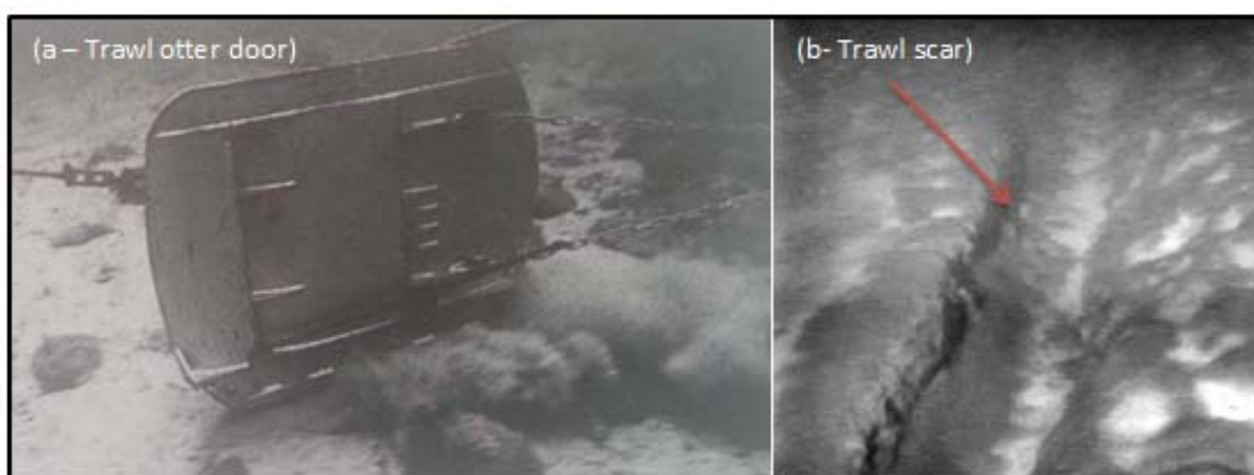
Figure 9: Typical indication of trawl door on the seabed (a); and trawl marks in soft seabed sediments (b); (Source: (a) Jennings et al. 2003; (b) Hopkins 2003).
