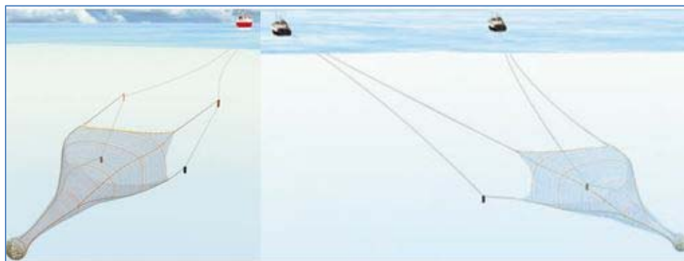
Figure 4: Typical configuration for pelagic trawl, single vessel (left) and paired vessels (right) – (Source: Galbraith and Rice, 2004).
