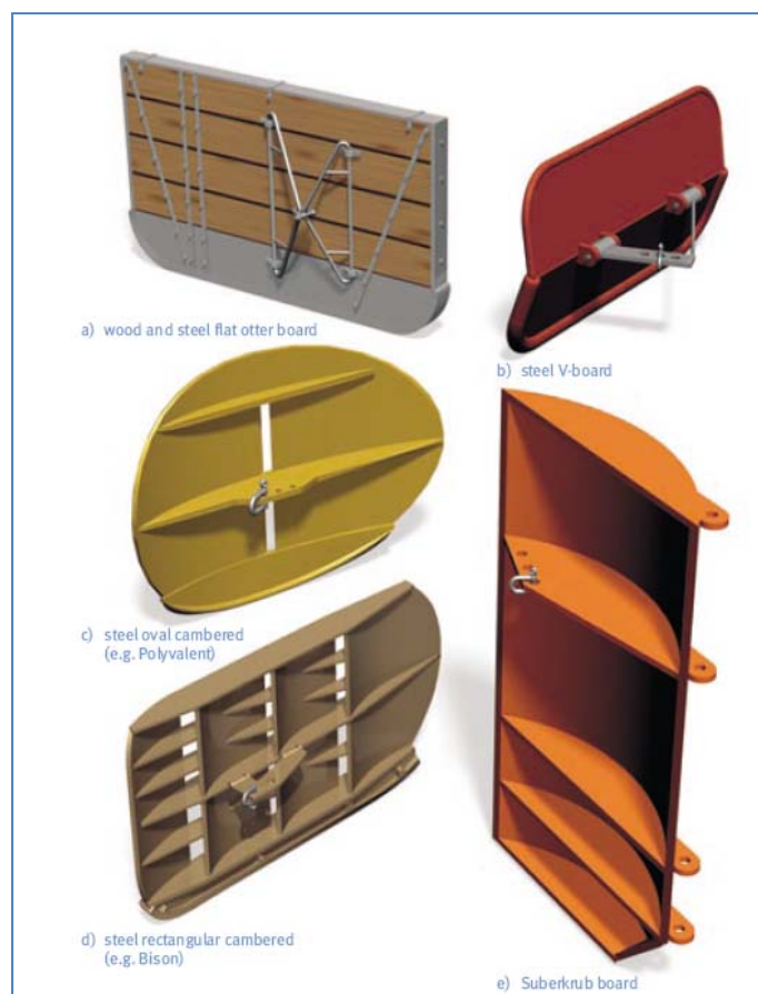
Figure 8: Typical otter board designs found on demersal trawls (Source: Galbraith and Rice, 2004).
