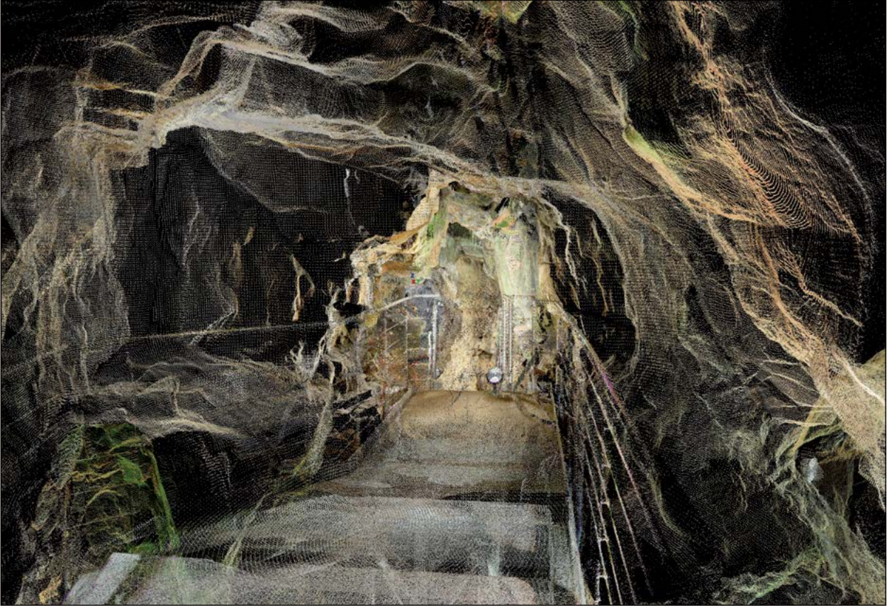
Fig.5.2. Laser technology provides a highly accurate and cost-effective tool for the surveying of subterranean features, as demonstrated by this unprocessed point cloud image of the interior of Church Hole cave. Photograph © Trent & Peak Archaeology
