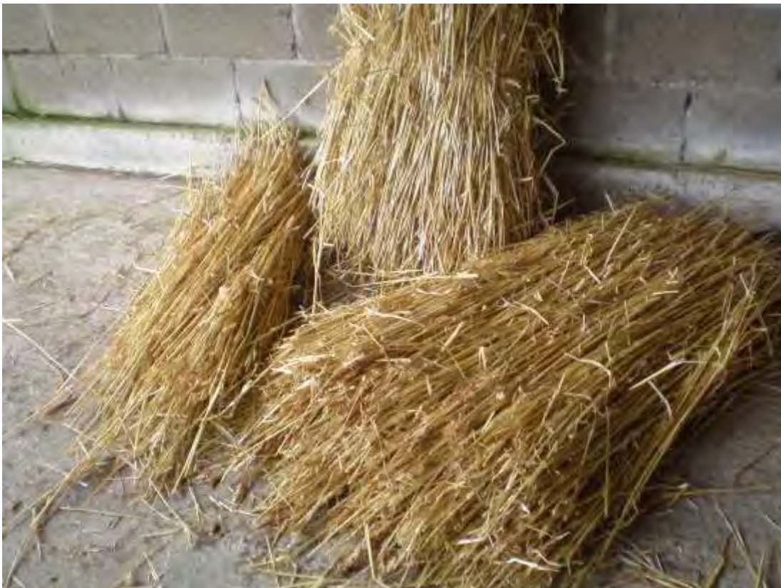
Above: Relatively undamaged threshed long straw, trussed bolt, yealm and sample of bolt. Very little waste!
