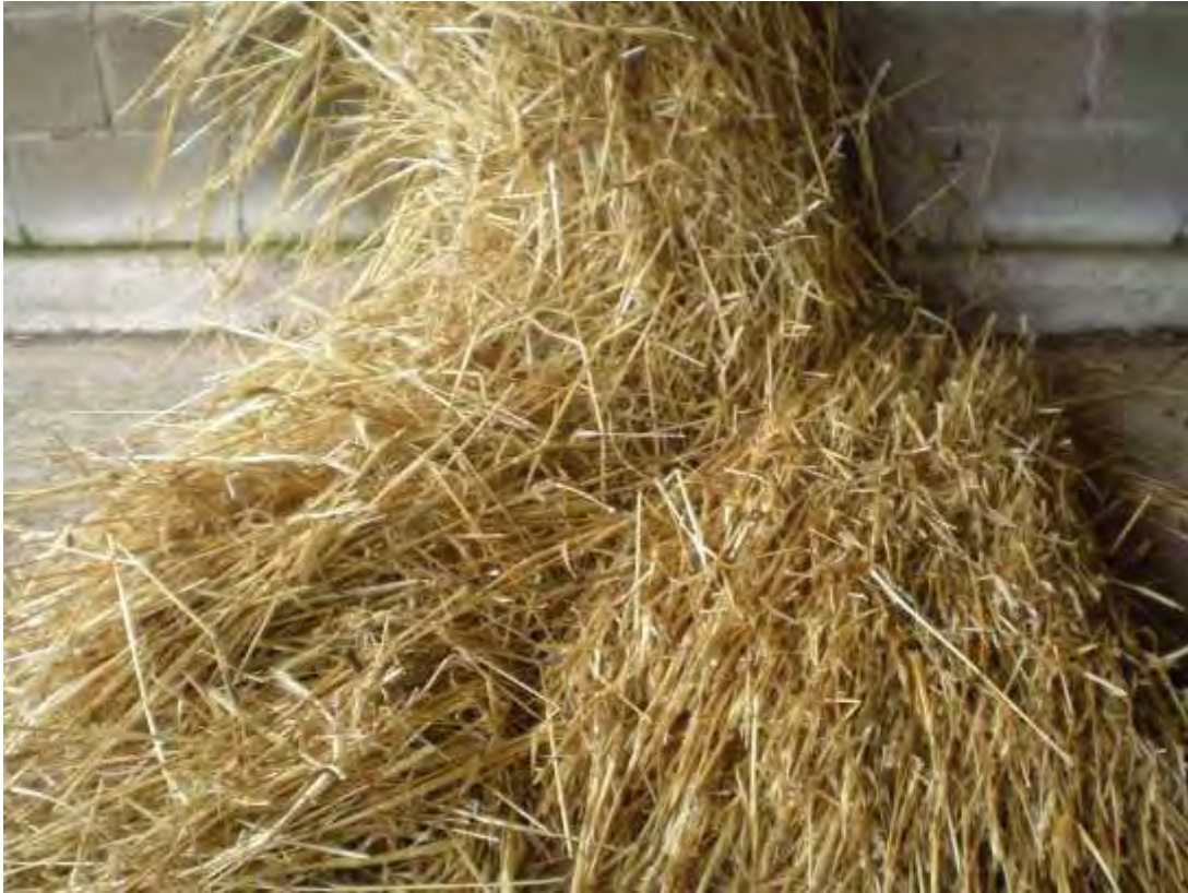
Above: Mechanically damaged long straw trussed bolt, yealm and waste.
