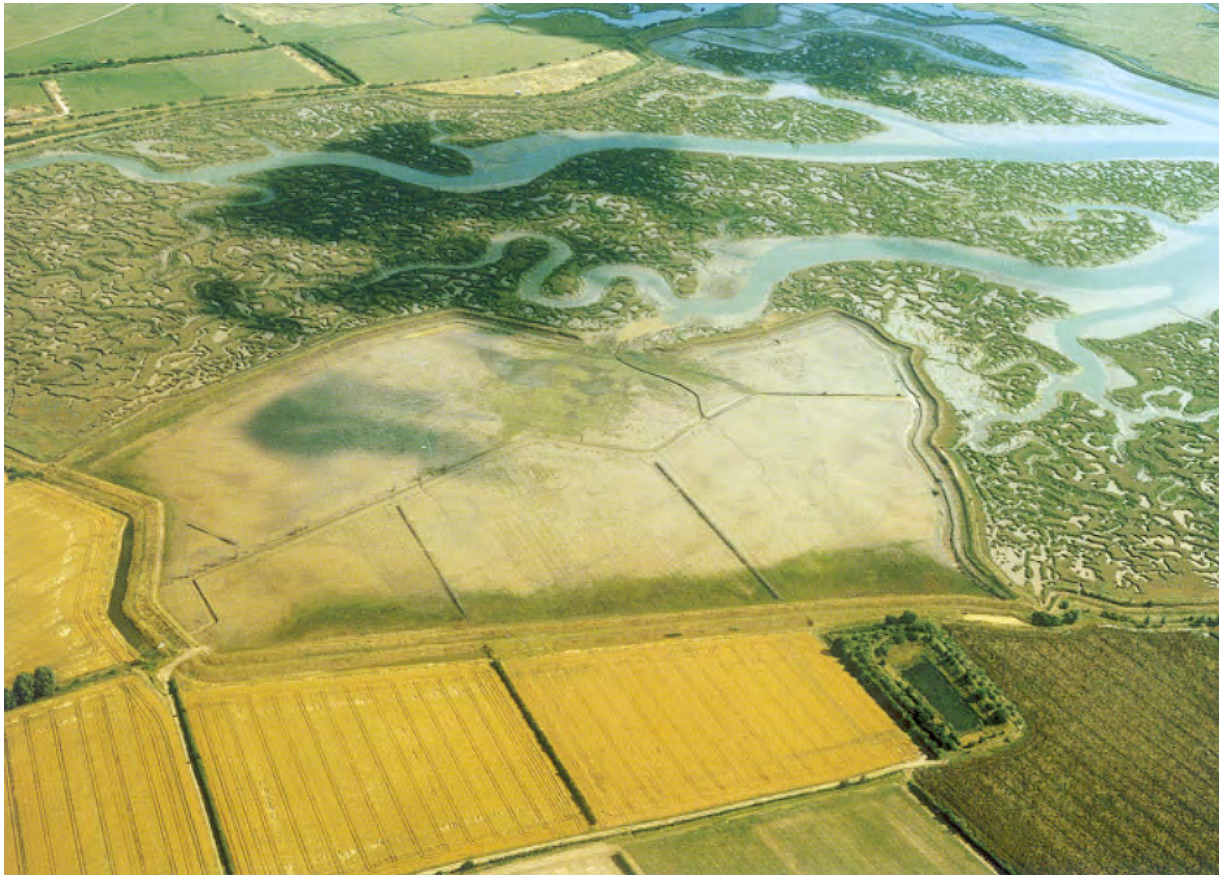
Fig. 24 An area of early managed realignment at Tollesbury. A number of red hills were recorded in the area prior to breaching the sea wall in 1995
