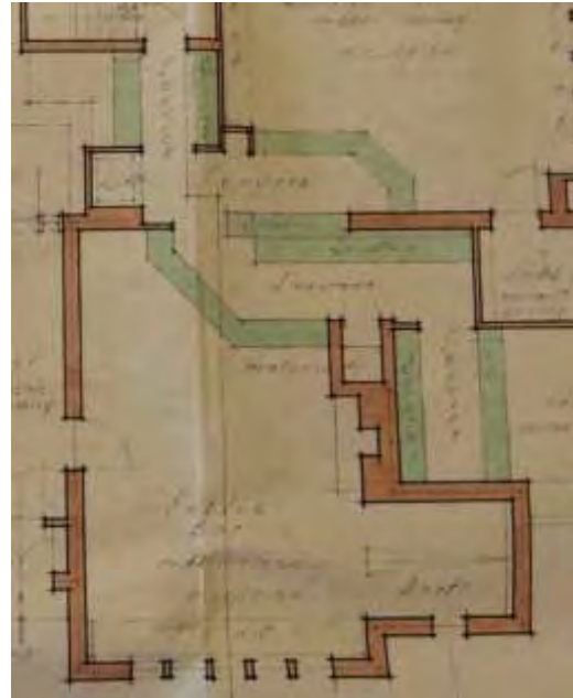
Hartcliffe Inn, Brocks Road, Hartcliffe. Detail of ground floor plan, 1959 and Red Hart, Bishport Avenue, Hartcliffe. Detail of ground floor plan showing diagonal staggered service space. © Bristol Record Office – BRO 29053/4c
