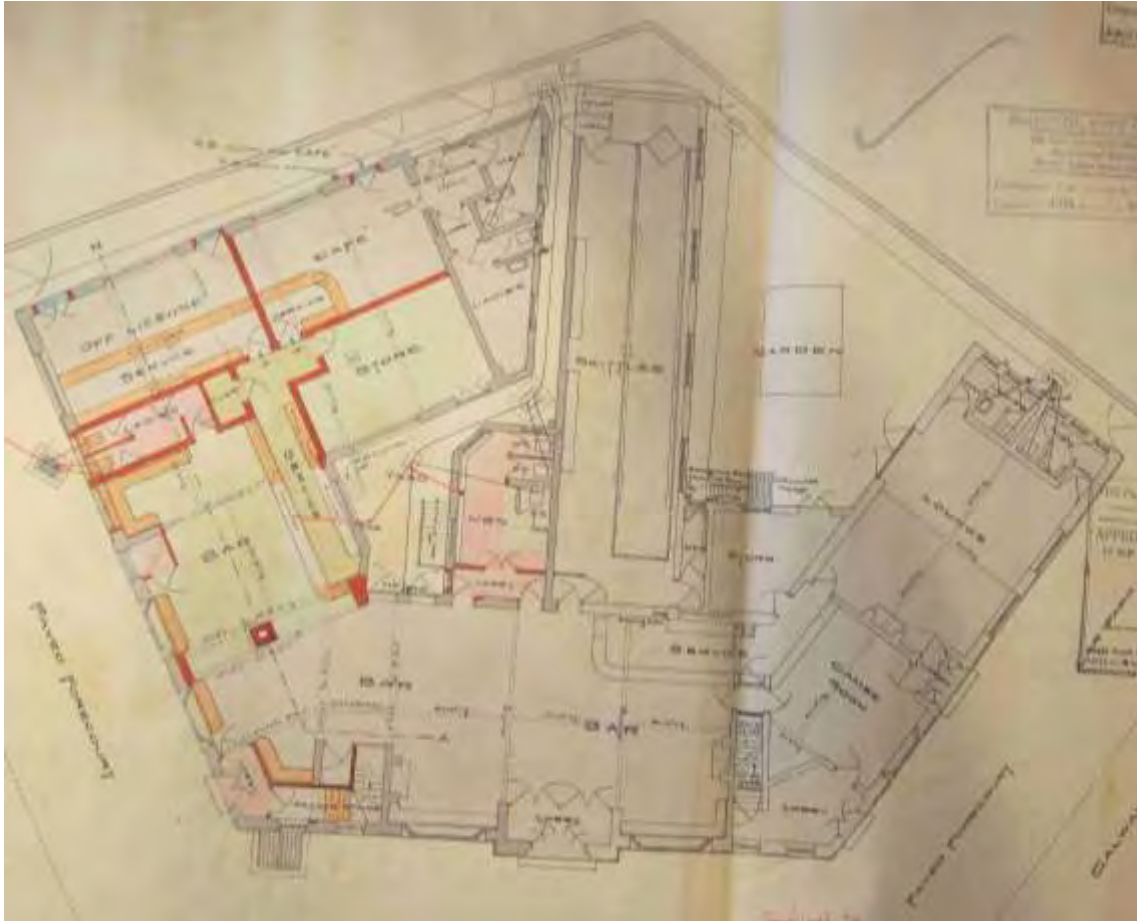
Plan showing proposed alterations to the ground floor of The Venture Inn, Melvin Square, Filwood Park, dated 3 May 1939 © Bristol Record Office – BRO 178/f64
