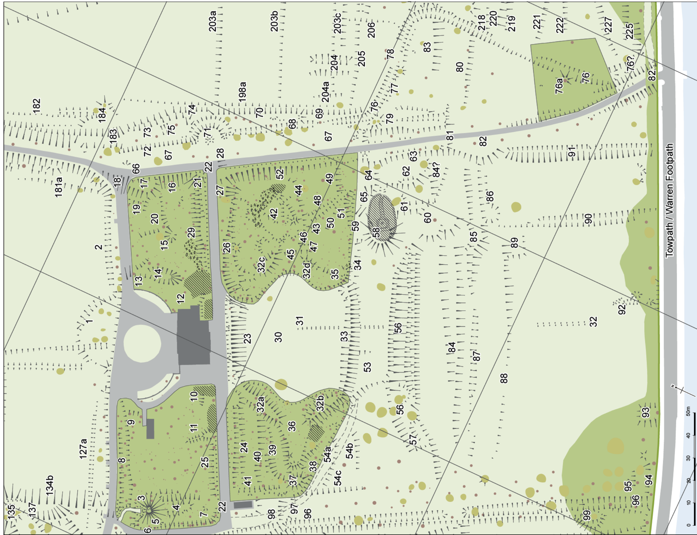
Figure 41 – Earthwork survey of the Pleasure Ground (1:1000@A3)
