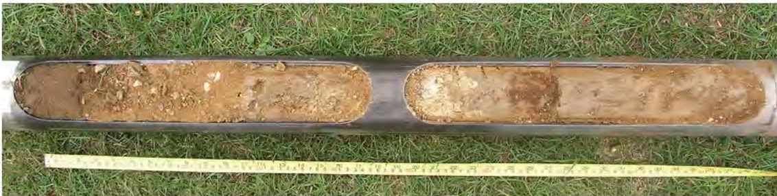
Figure 175 Core B. Probably gravel over natural clay at ca. 26cm
