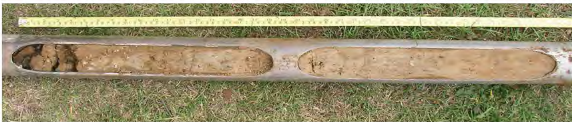
Figure 177 Core C2. Core C shows 2 m depth of heavy clay suggesting this is natural geology
