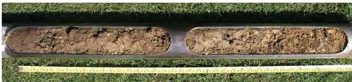
Figure 182 Core H. 45/50 looks like a make-up layer
