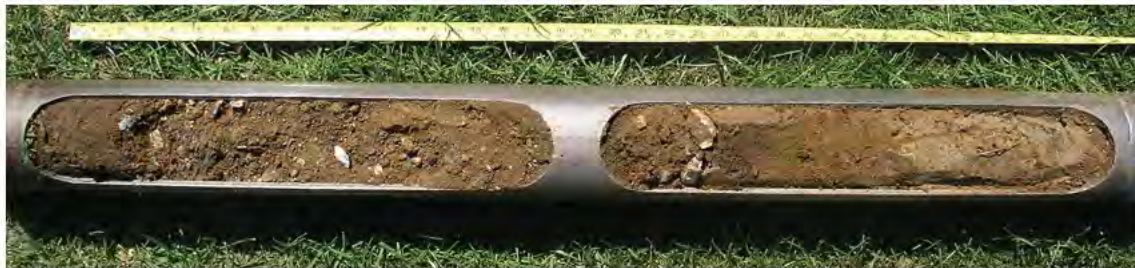
Figure 181 Core G. Gravel on compacted buried topsoil at 57/60 - 63/66. ?On top of dam make-up layer or dredgings
