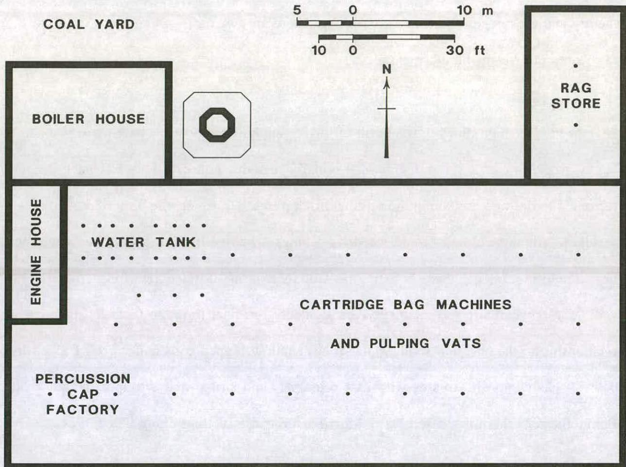
Building 17: Diagrammatic ground plan reconstructing original layout (based on PRO, WORK 43/1615)
