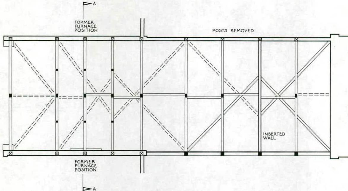
PLAN OF CENTRAL ROOF AT TIE BEAM LEVEL WITH CROSS BRACING RECONSTRUCTED AND POST POSITIONS BELOW INDICATED
