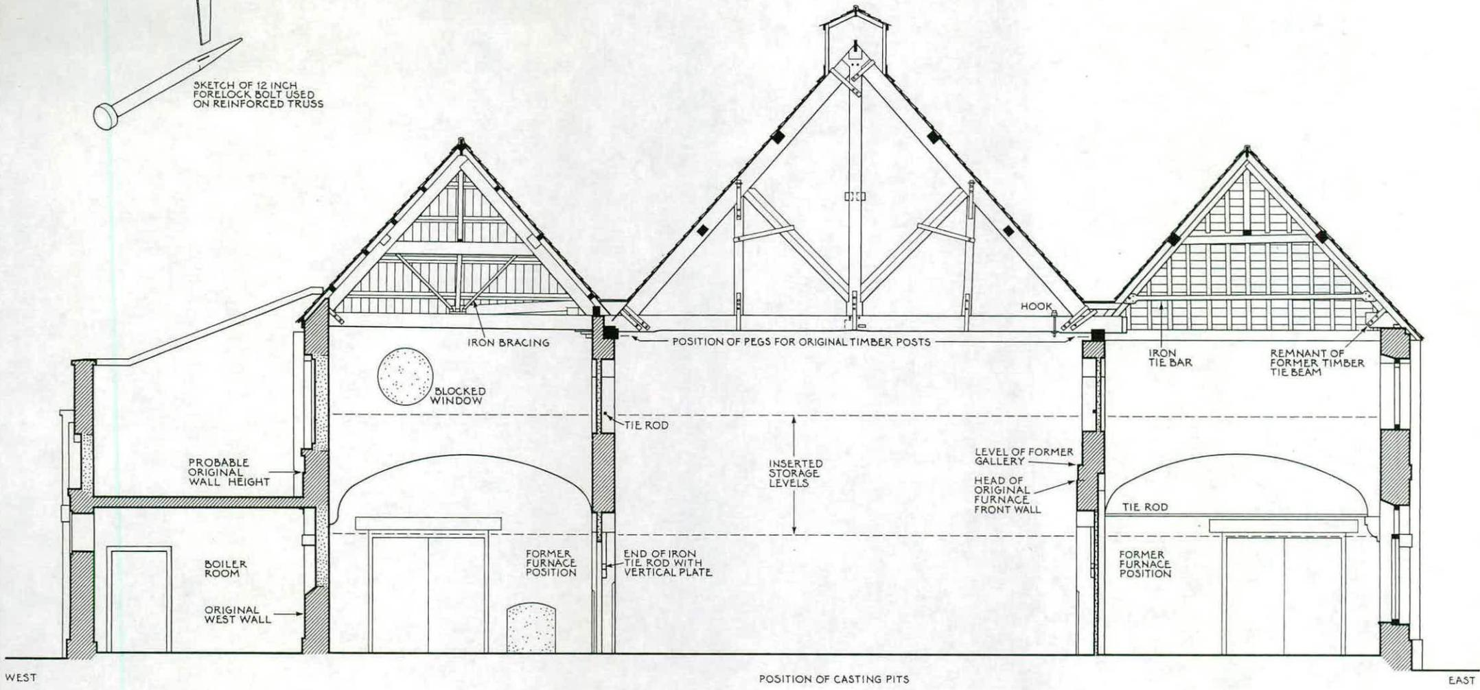
SECTION A-A THROUGH FURNACE AND CASTING PIT POSITIONS SHOWING REINFORCED ROOF TRUSS
