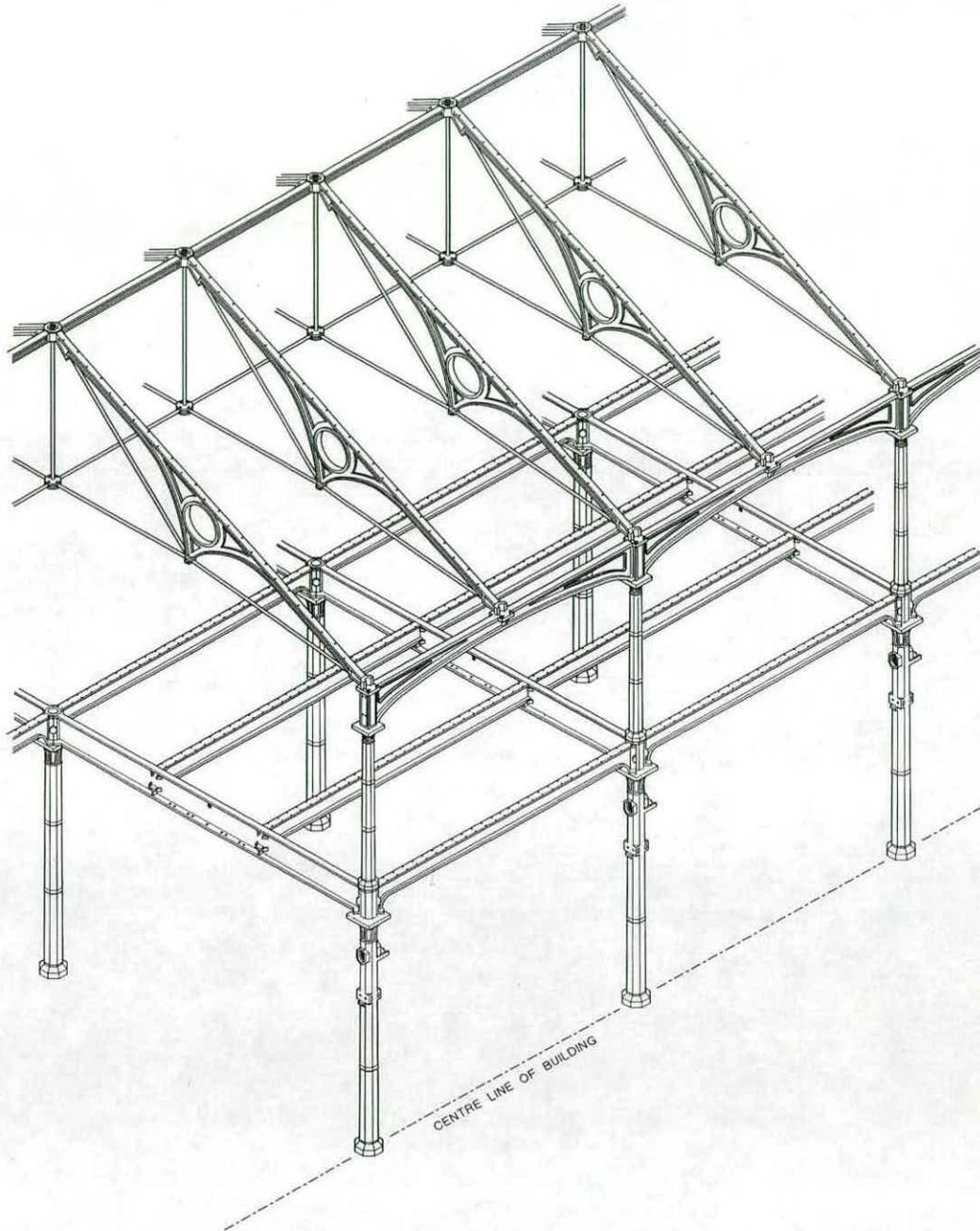
ISOMETRIC VIEW OF TWO BAYS OF INTERNAL IRON FRAME
