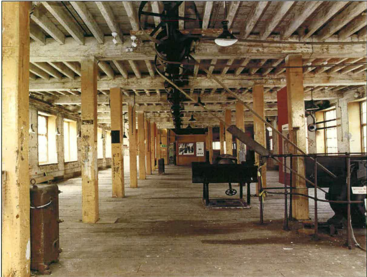
Figure 17. The first floor of the north range of the wood mills in 2003 showing the overhead power transmission. The Lignum vitae saw is off the picture to the right. [AA042411]
