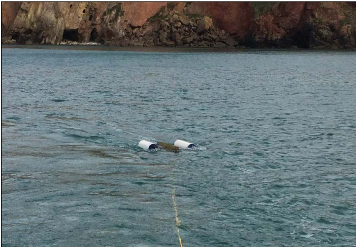
Fig. 4: Magnetometer and float arrangement towed behind the vessel
