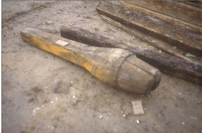
Photograph 6: 'Tampion' valve plug, removed during works at Elton Reservoir
