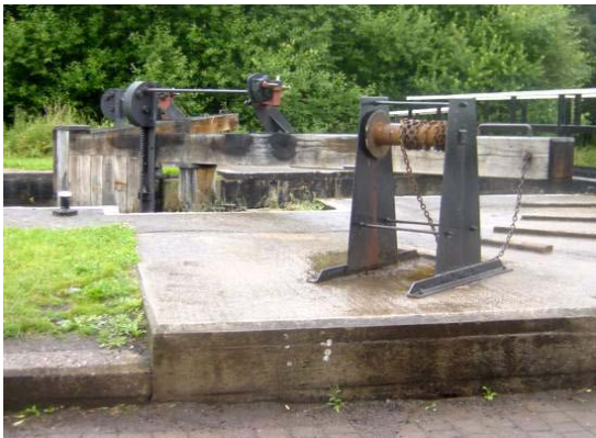
Chain-operated balance beam, lower Poolstock Lock. ( www.penninewaterways.co.uk )
