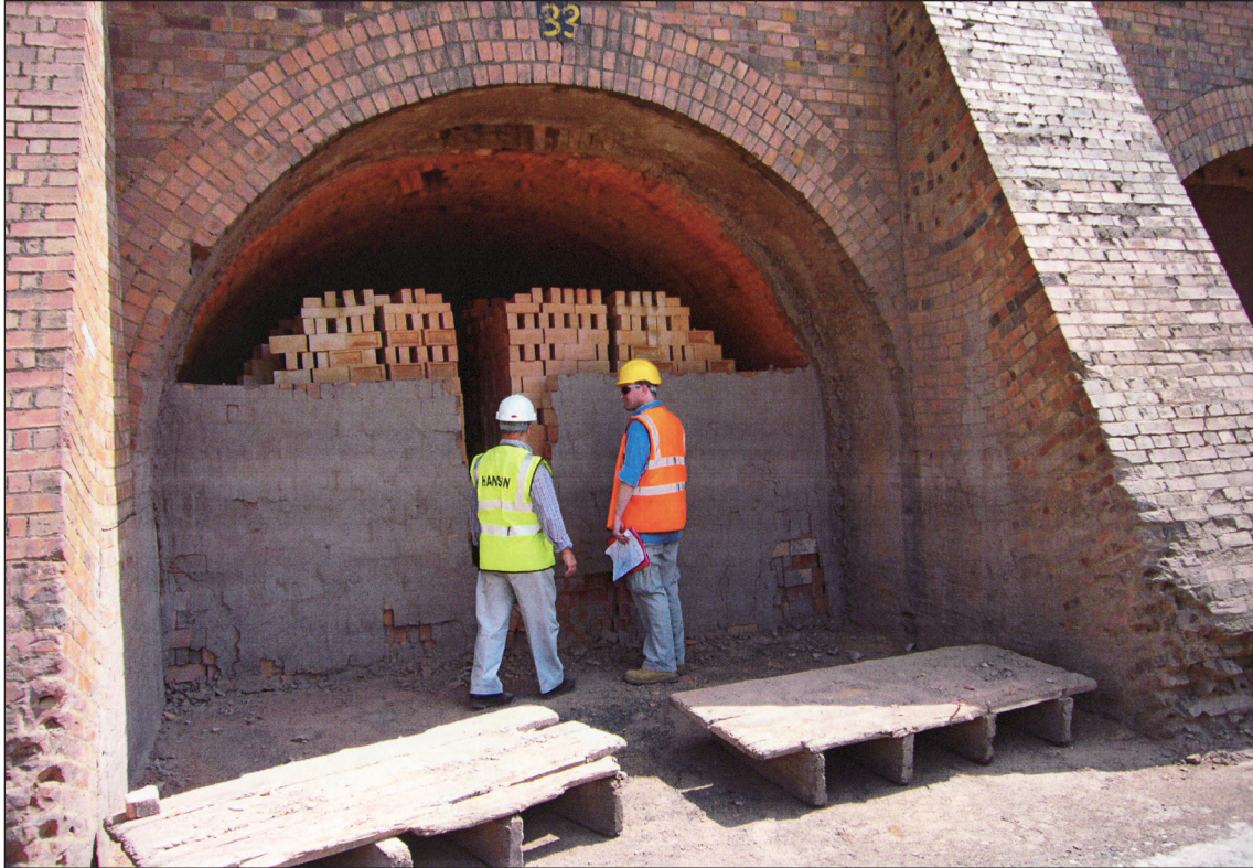
Figure 15 CK3, fired bricks in chamber © Historic England
