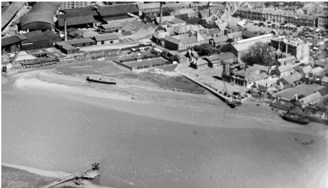
Fig. 20 An aerial view of the Common Staithe from the south-west in 1930, showing how the foreshore had silted up, leaving only the southernmost part of the quay in use. Detail of HEA (Aerofilms Collection) EPW031687 1930.
